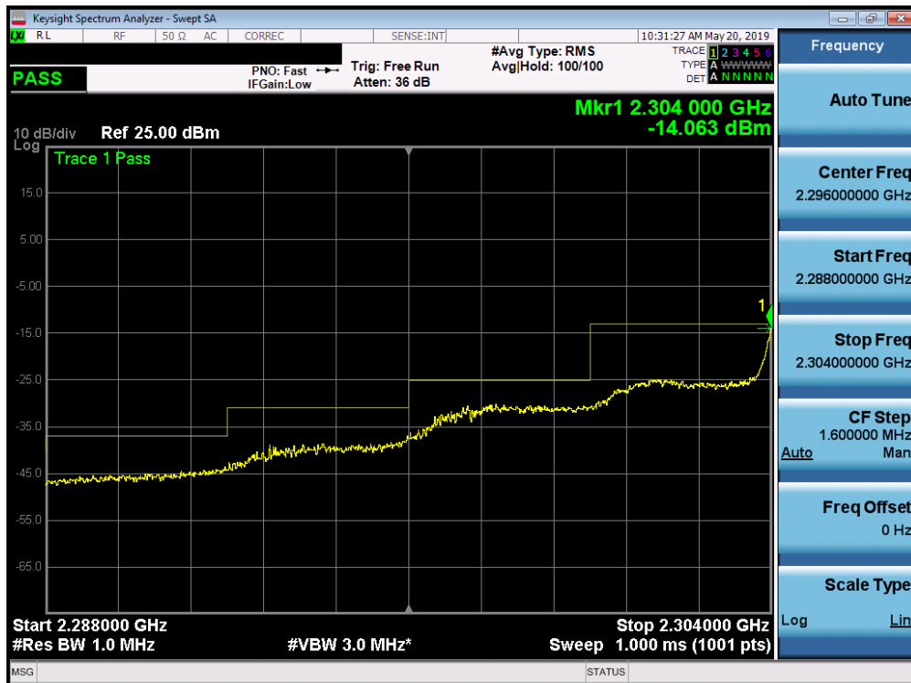
Plot 7-161. Lower Extended Band Edge Plot (Band 30 - 5.0MHz QPSK - Full RB Configuration)
