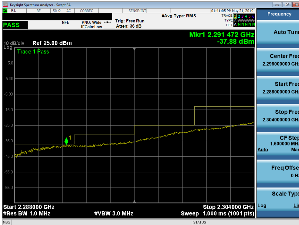
Plot 7-165. Lower Extended Band Edge Plot (Band 30 - 10.0MHz QPSK - Full RB Configuration)
