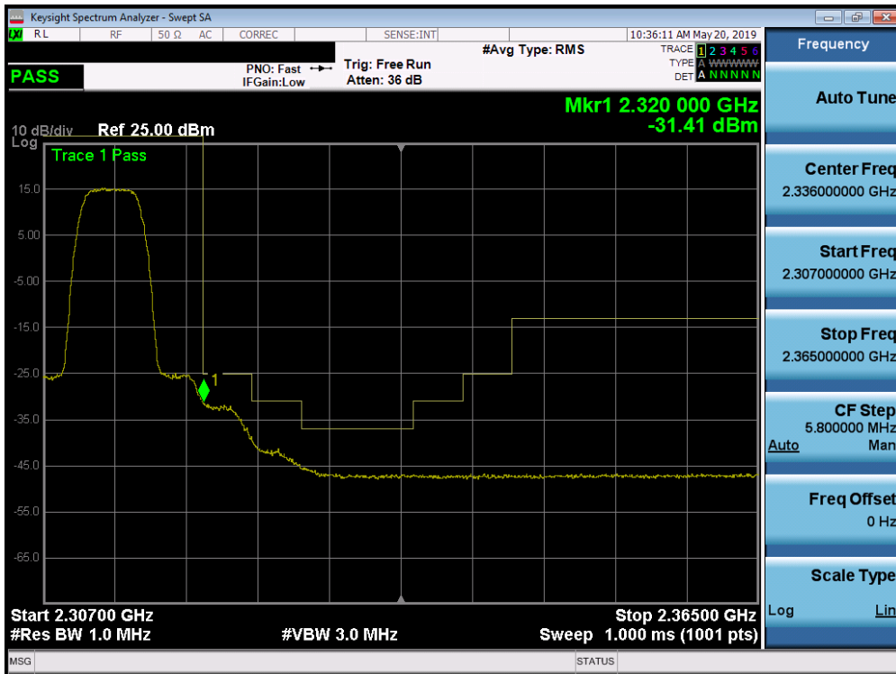
Plot 7-163. Upper Extended Band Edge Plot (Band 30 - 5.0MHz QPSK - Full RB Configuration)
