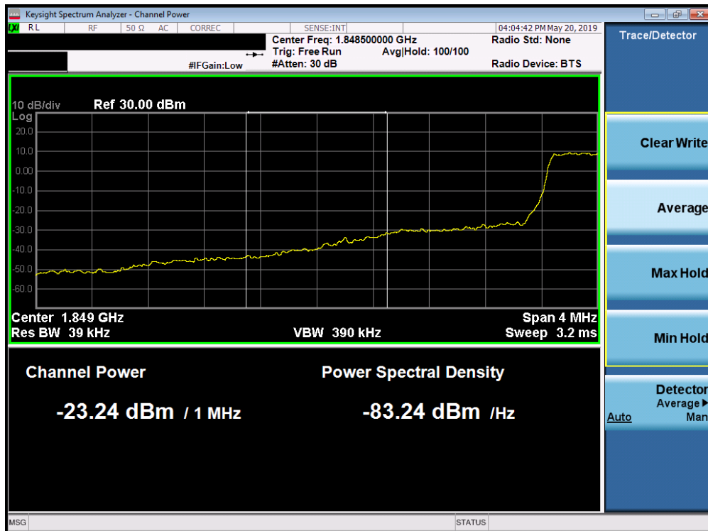
Plot 7-137. Lower Extended Band Edge Plot (Band 2 - 1.4MHz QPSK - Full RB Configuration)
