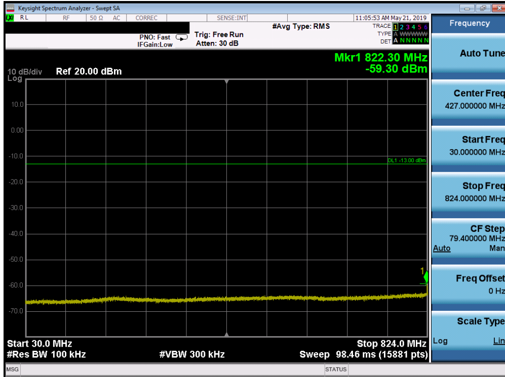
Plot 7-60. Conducted Spurious Plot (Band 5 - 10.0MHz QPSK - RB Size 1, RB Offset 0 - High Channel)
