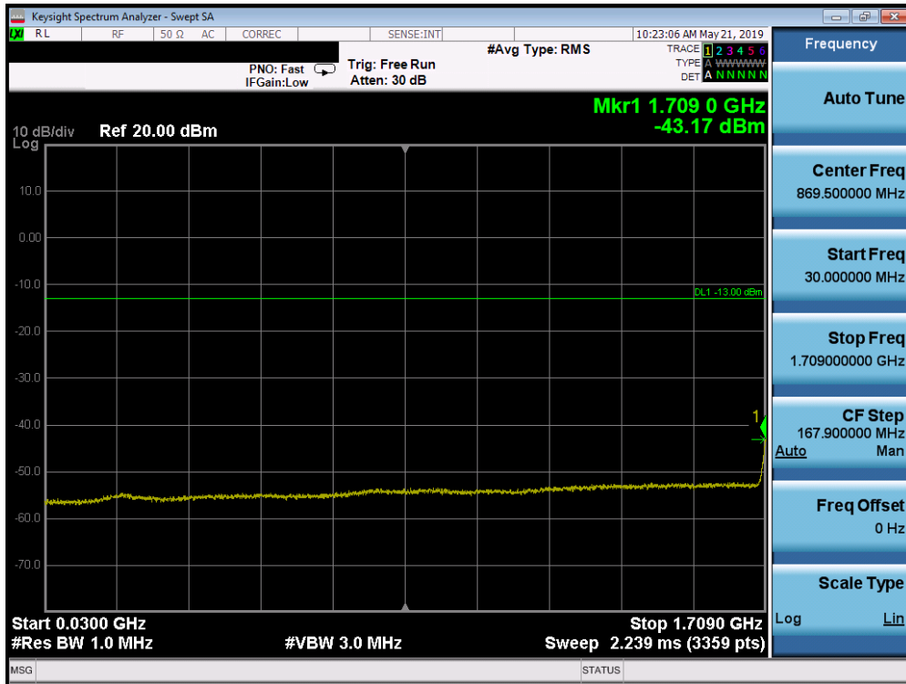
Plot 7-63. Conducted Spurious Plot (Band 66/4 - 20.0MHz QPSK - RB Size 1, RB Offset 0 - Low Channel)
