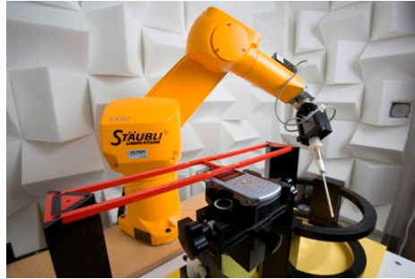
Figure 4-3 SPEAG Robotic System
