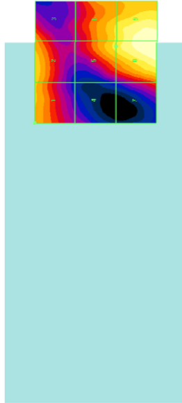
Figure 9-1 Sample E-field Scan Overlay (See Test Setup Photographs for actual WD overlay)
