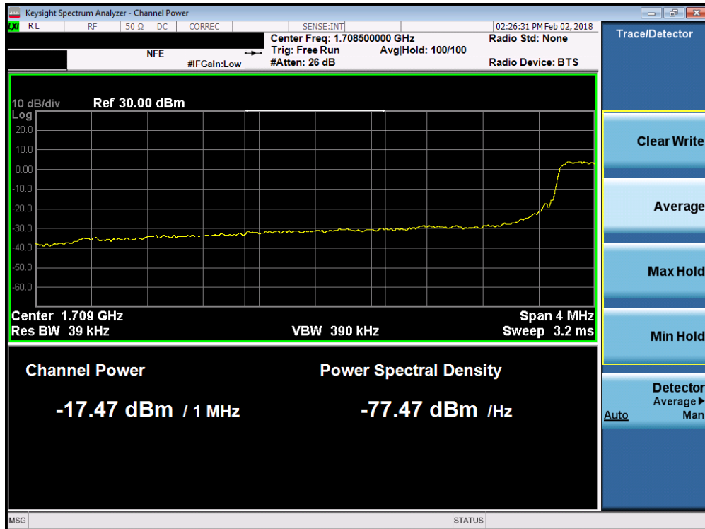
Plot 6-98. Lower Extended Band Edge Plot (Band 4 - 5.0MHz QPSK - Full RB Configuration)
