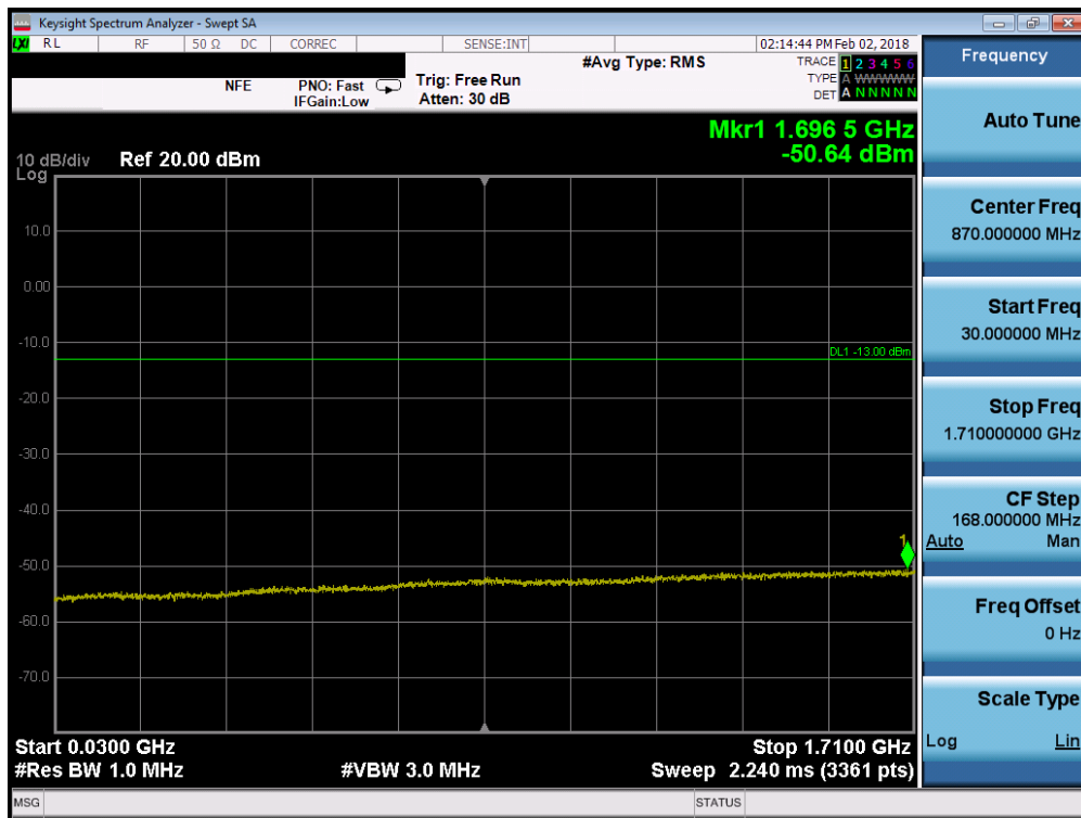
Plot 6-58. Conducted Spurious Plot (Band 4 - 1.4MHz QPSK - RB Size 1, RB Offset 0 - Mid Channel)
