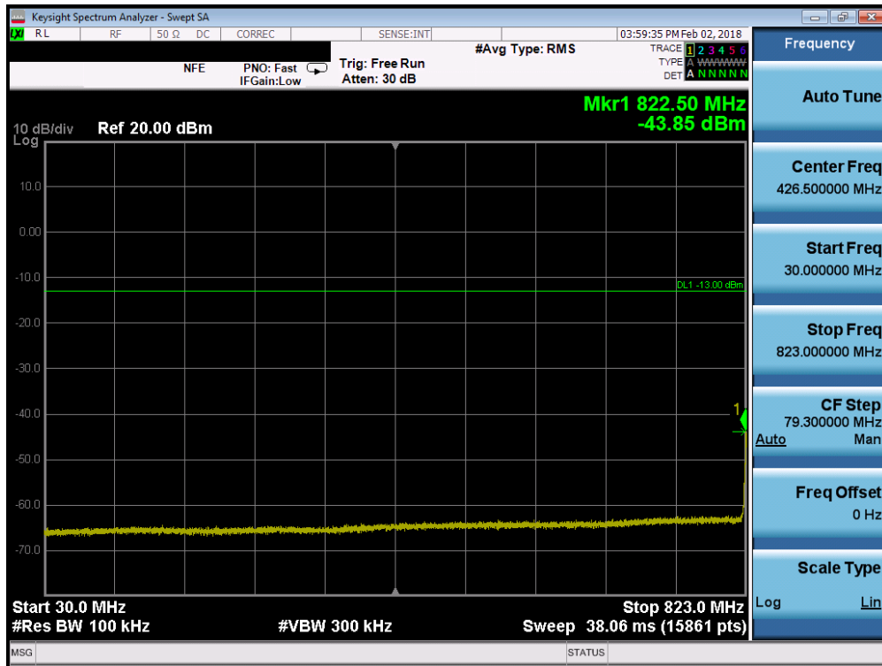
Plot 6-46. Conducted Spurious Plot (Band 5 - 1.4MHz QPSK - RB Size 1, RB Offset 0 - Low Channel)
