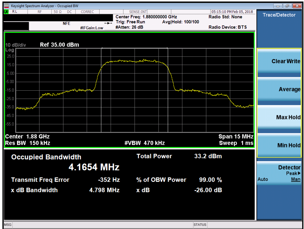
Plot 7-8. Occupied Bandwidth Plot (PCS WCDMA Mode)
