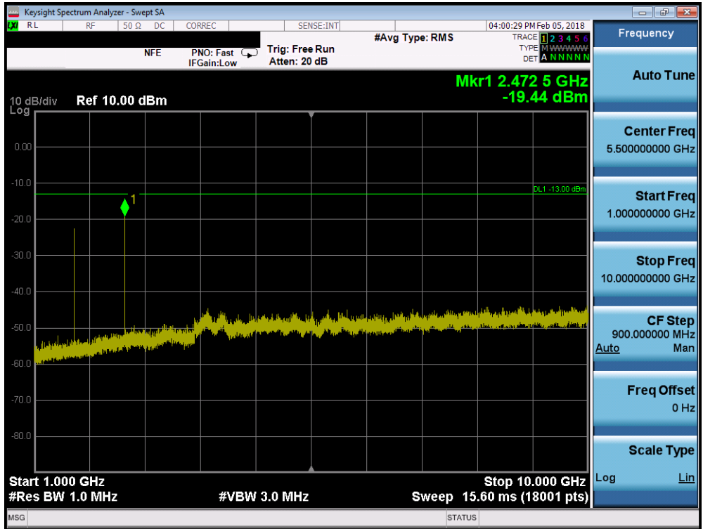
Plot 7-11. Conducted Spurious Plot (Cellular GPRS Mode - Low Channel)
