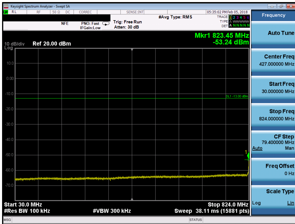
Plot 7-48. Conducted Spurious Plot (Cellular WCDMA Mode - Mid Channel)
