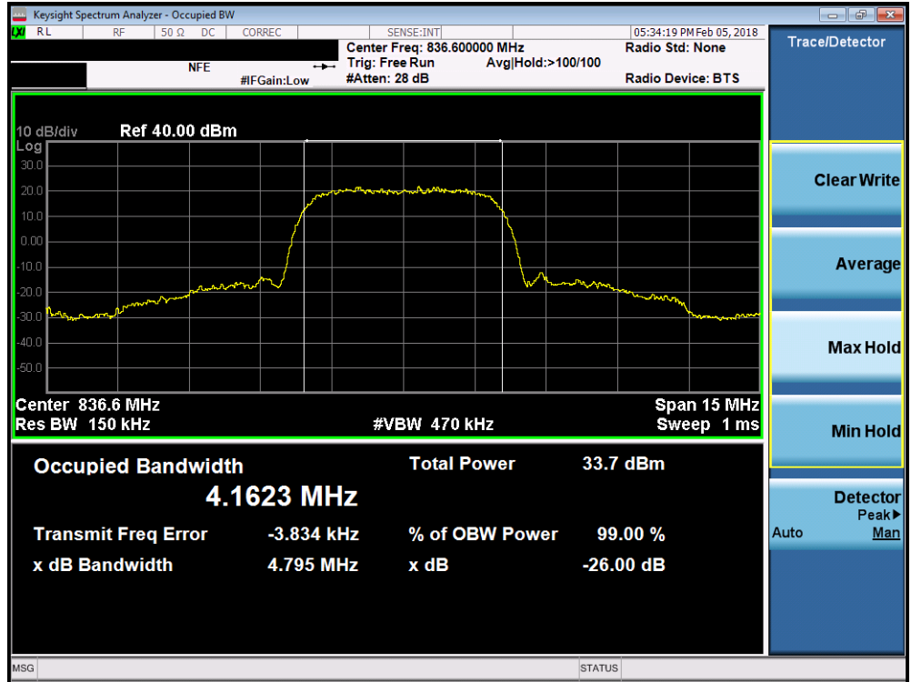
Plot 7-7. Occupied Bandwidth Plot (Cellular WCDMA Mode)
