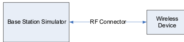
Figure 9-2 Power Measurement Setup
