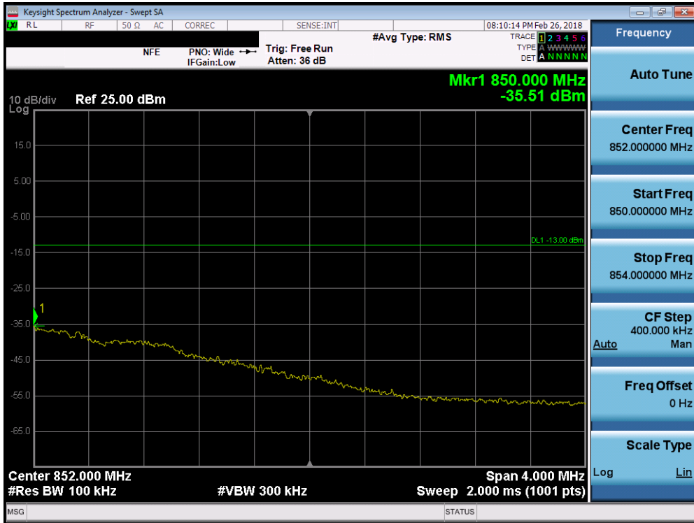
Plot 7-126. Upper Extended Band Edge Plot (Band 5 - 1.4MHz QPSK - Full RB Configuration)
