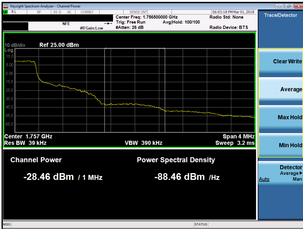
Plot 7-136. Upper Extended Band Edge Plot (Band 4 - 1.4MHz QPSK - Full RB Configuration)
