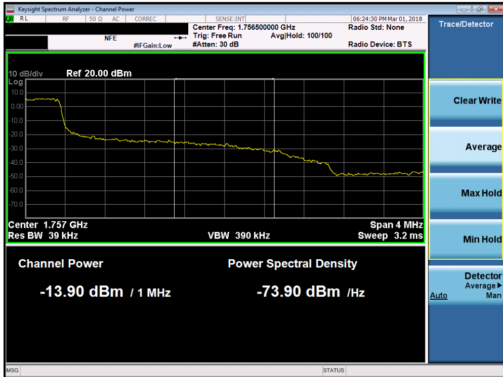
Plot 7-142. Upper Extended Band Edge Plot (Band 4 - 3.0MHz QPSK - Full RB Configuration)
