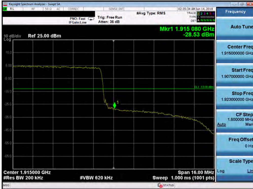
Plot 7-211. Upper Band Edge Plot (Band 25 - 20.0MHz QPSK - Full RB Configuration)
