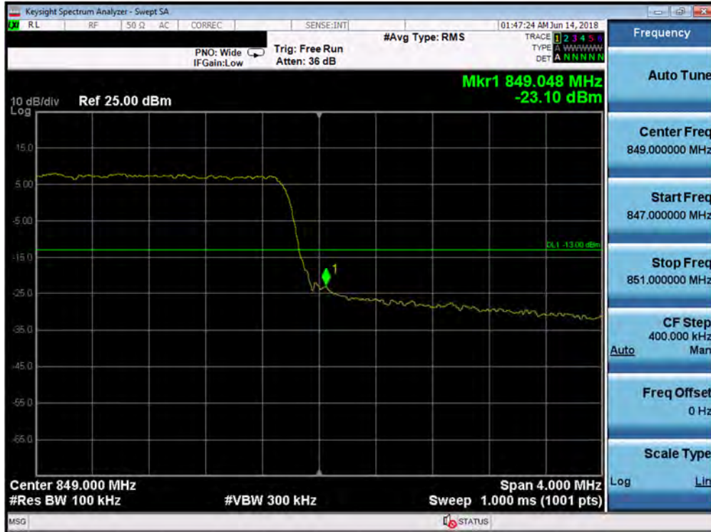
Plot 7-148. Upper Band Edge Plot (Band 26/5 - 5.0MHz QPSK - Full RB Configuration)
