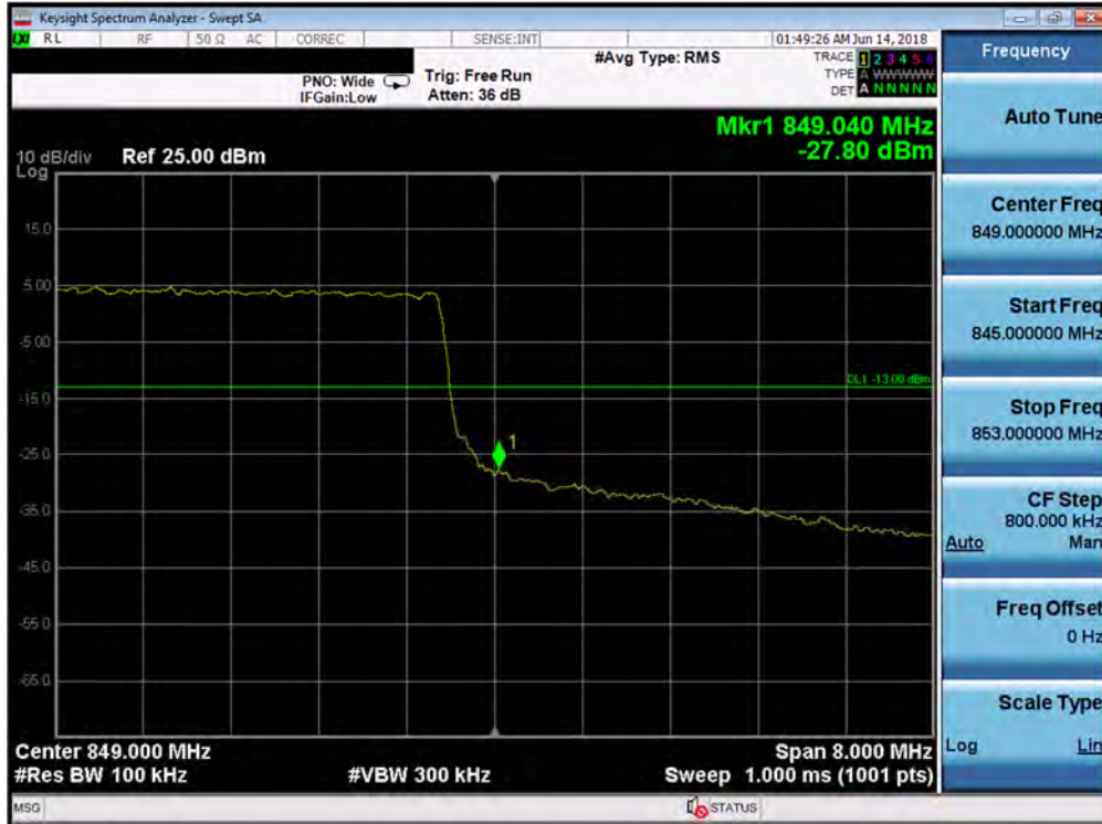
Plot 7-150. Upper Band Edge Plot (Band 26/5 - 10.0MHz QPSK - Full RB Configuration)
