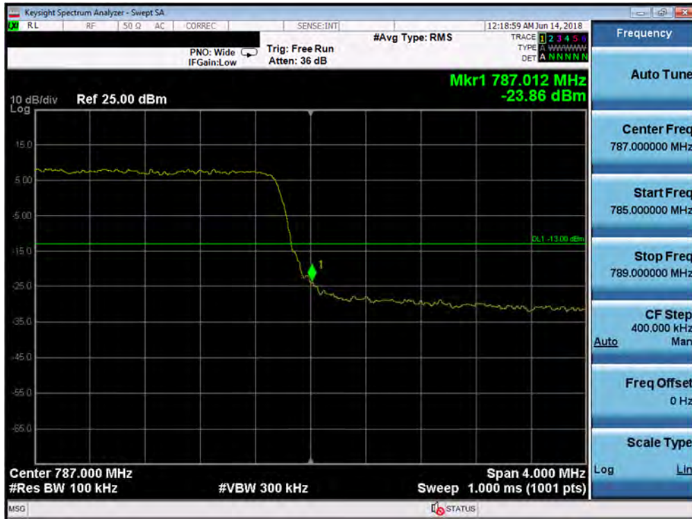
Plot 7-136. Upper Band Edge Plot (Band 13 - 5.0MHz QPSK - Full RB Configuration)
