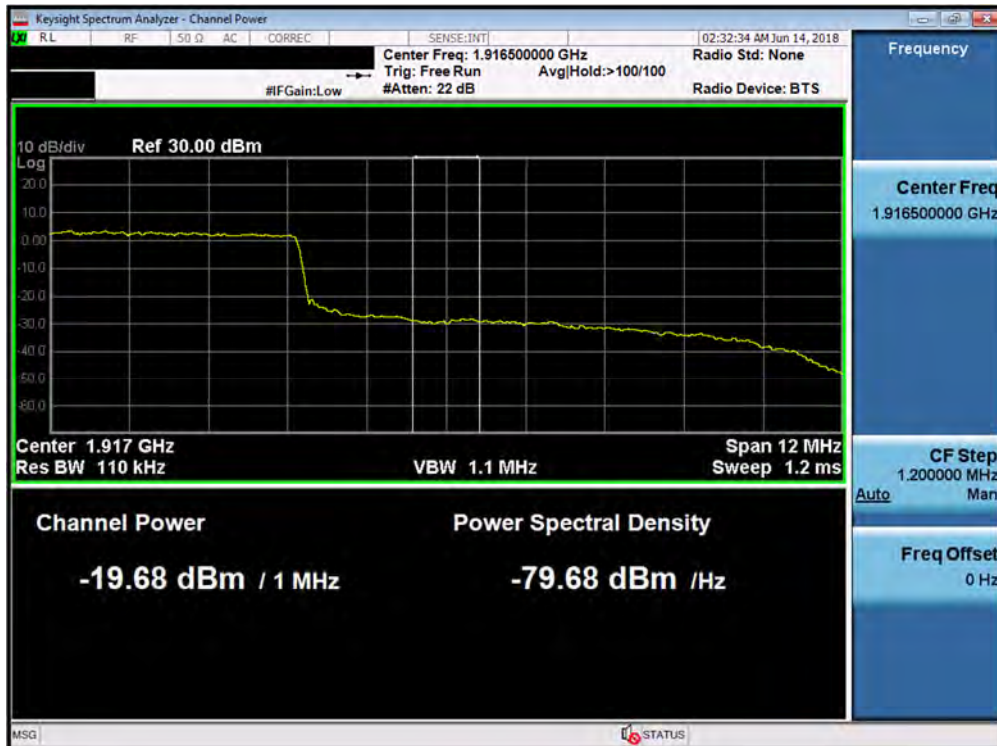
Plot 7-206. Upper Extended Band Edge Plot (Band 25 - 15.0MHz QPSK - Full RB Configuration)
