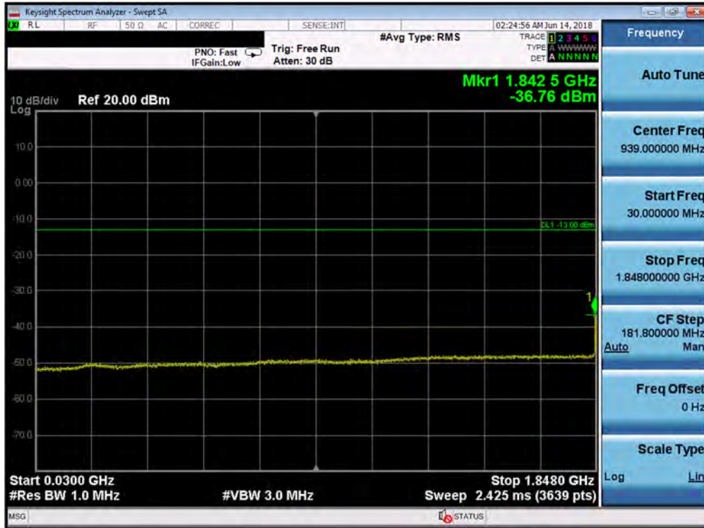
Plot 7-99. Conducted Spurious Plot (Band 25/2 - 5.0MHz QPSK - RB Size 1, RB Offset 0 - Low Channel)
