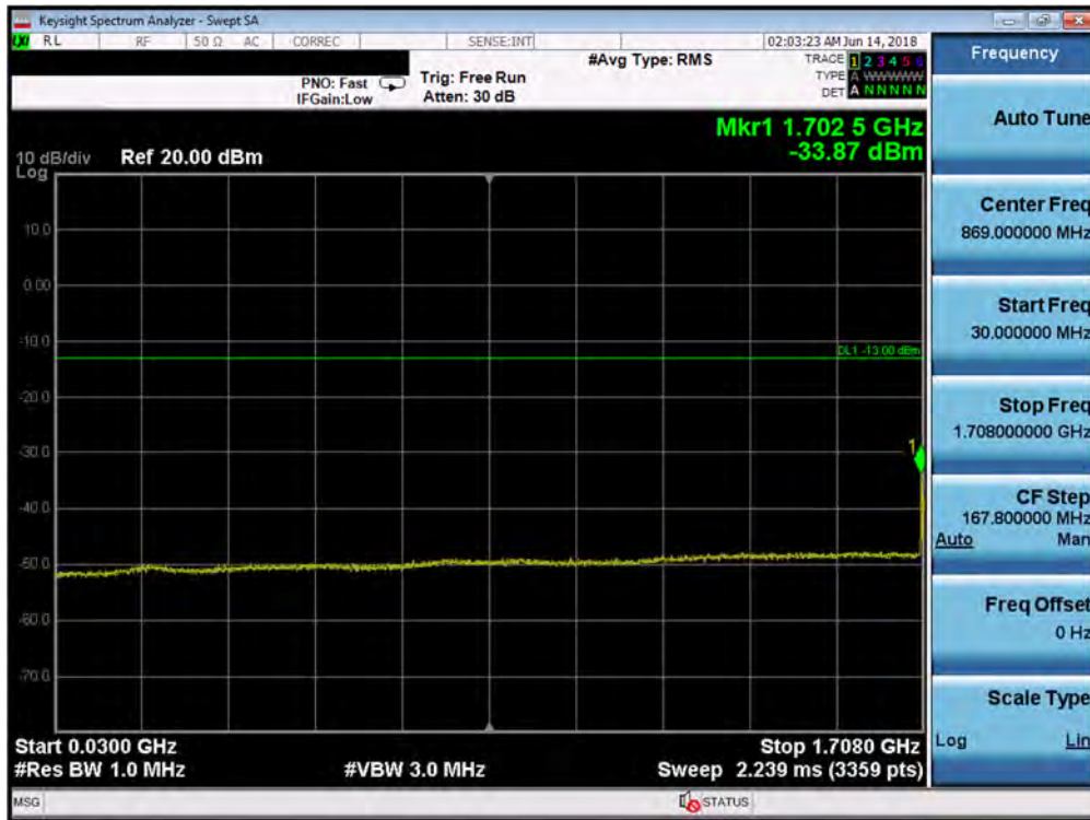
Plot 7-90. Conducted Spurious Plot (Band 4 - 5.0MHz QPSK - RB Size 1, RB Offset 0 - Low Channel)
