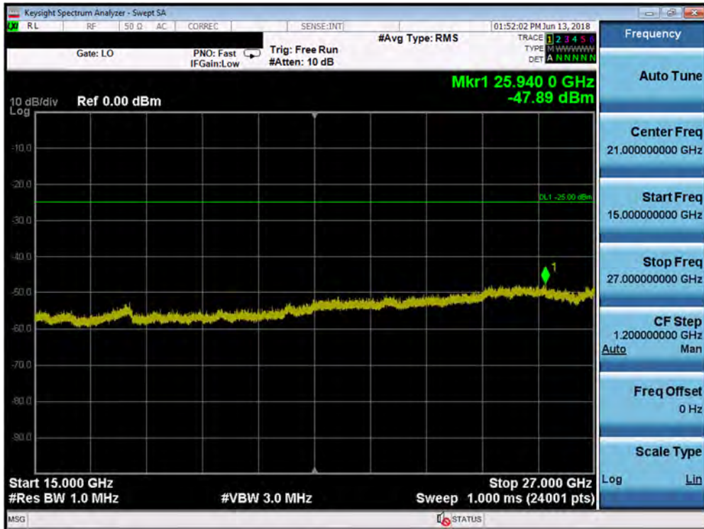
Plot 7-122. Conducted Spurious Plot (Band 41 PC2 - 5.0MHz QPSK - RB Size 1, RB Offset 0 - Mid Channel)
