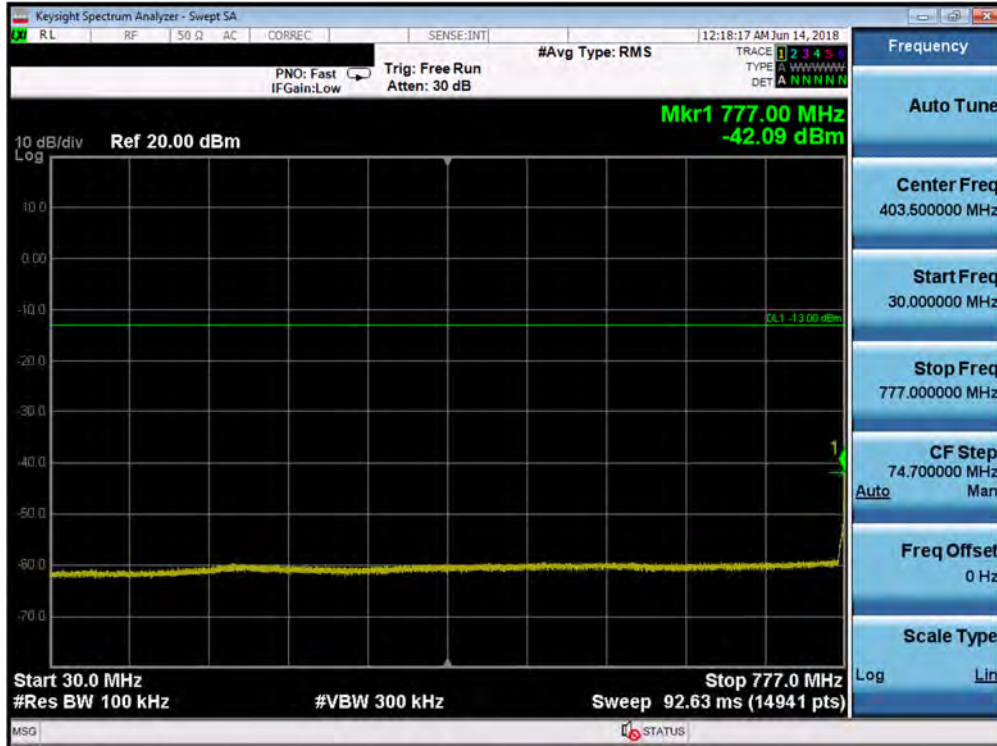
Plot 7-78. Conducted Spurious Plot (Band 13 - 5.0MHz QPSK - RB Size 1, RB Offset 0 - High Channel)
