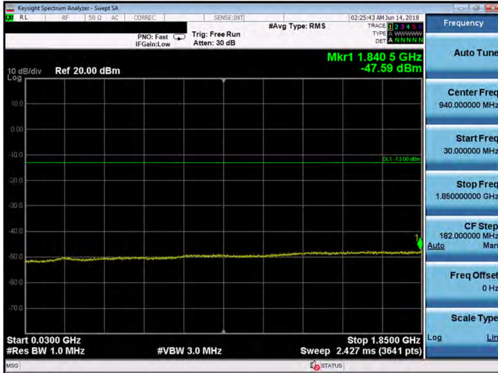
Plot 7-105. Conducted Spurious Plot (Band 25/2 - 5.0MHz QPSK - RB Size 1, RB Offset 0 - High Channel)
