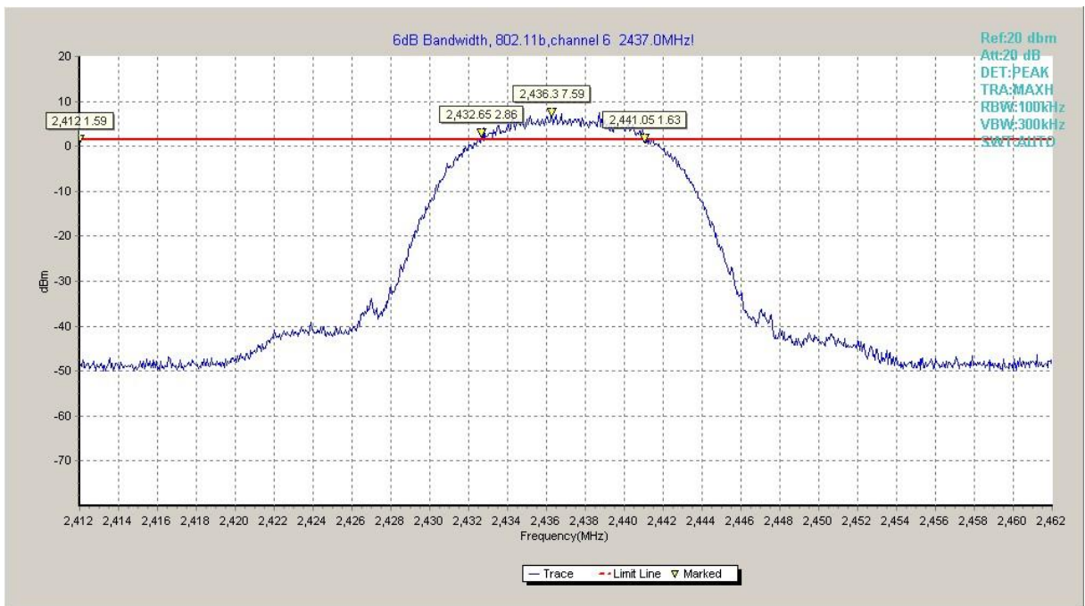
Fig.A.4.2 Occupied 6dB Bandwidth (802.11b, Ch 6)
