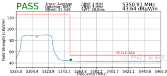
Plot 7-94. Radiated Upper Band Edge Plot SISO ANT1 (Average – UNII Band 2A)
