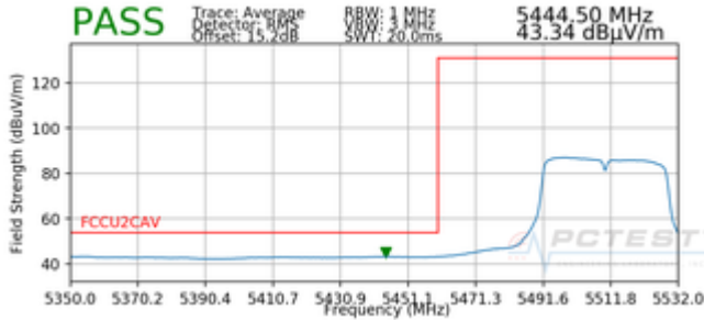
Plot 7-96. Radiated Lower Band Edge Plot SISO ANT1 (Average – UNII Band 2C)
