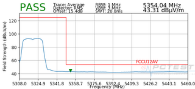
Plot 7-85. Radiated Upper Band Edge Plot SISO ANT1 (Average – UNII Band 2A)
