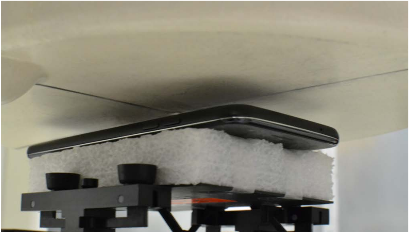
SAR Test Setup Photo 5 – Back Side at 10mm
