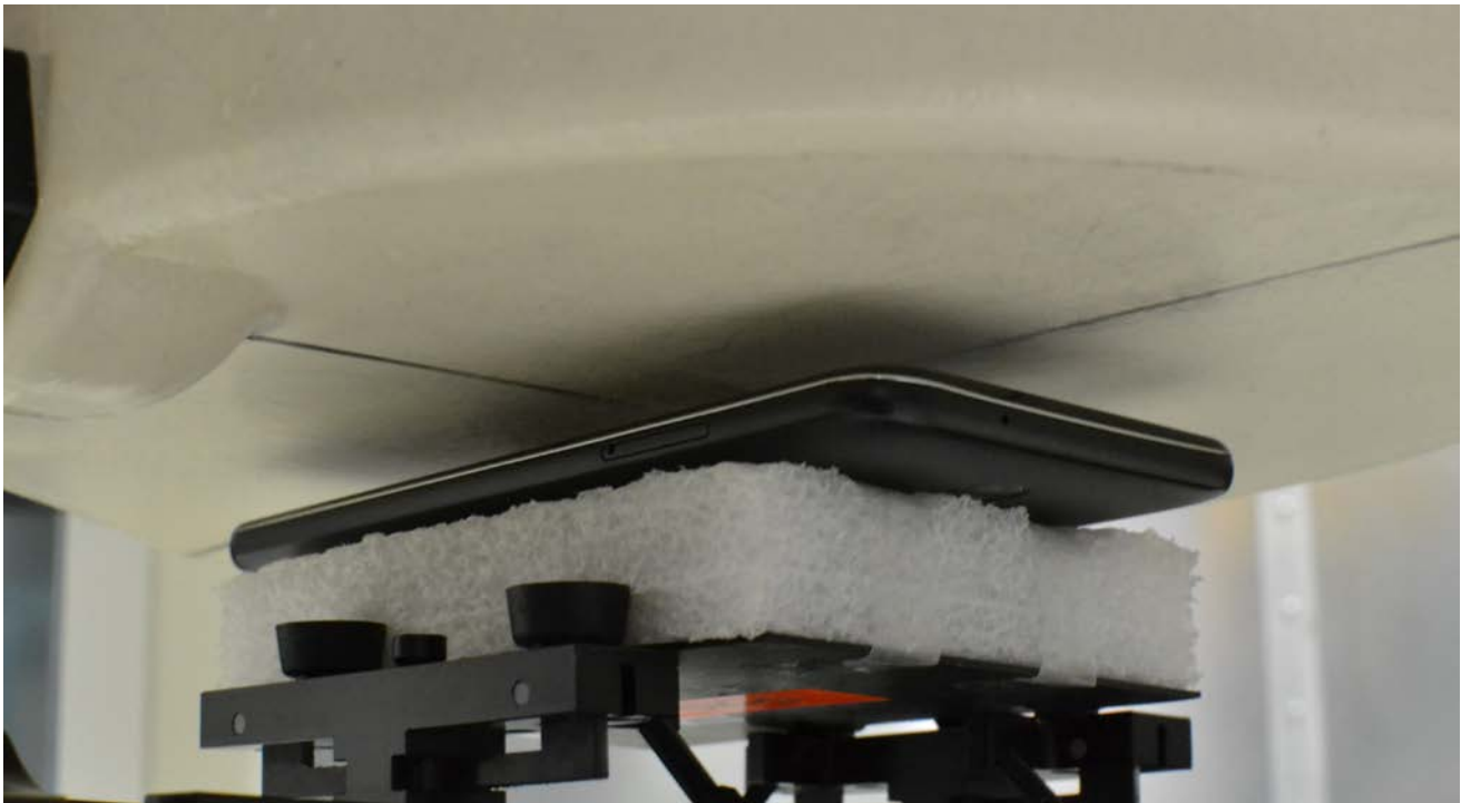
SAR Test Setup Photo 6 – Front Side at 10mm
