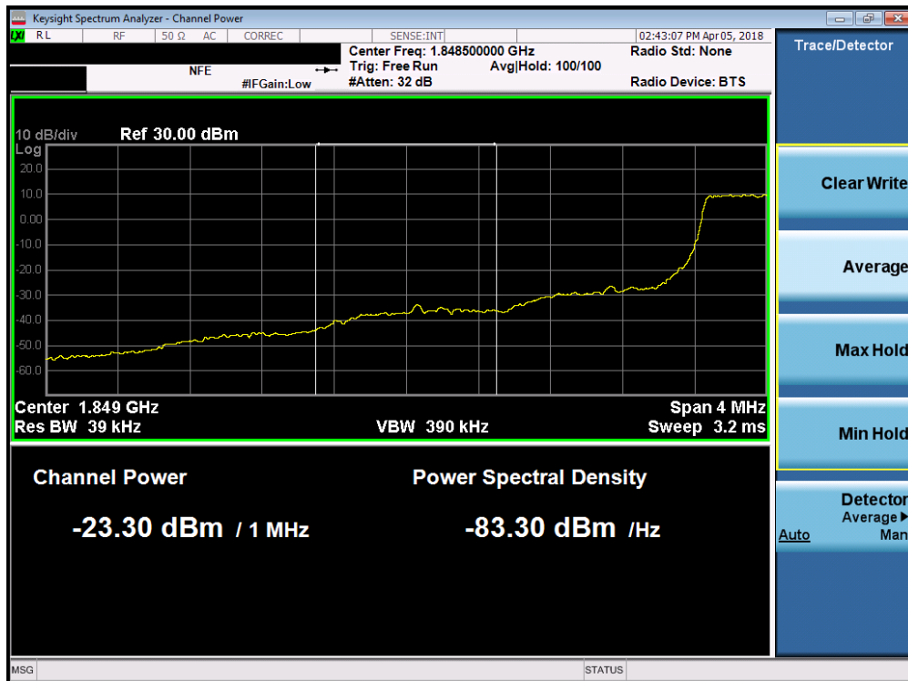
Plot 7-120. Lower Extended Band Edge Plot (Band 2 - 1.4MHz QPSK - Full RB Configuration)
