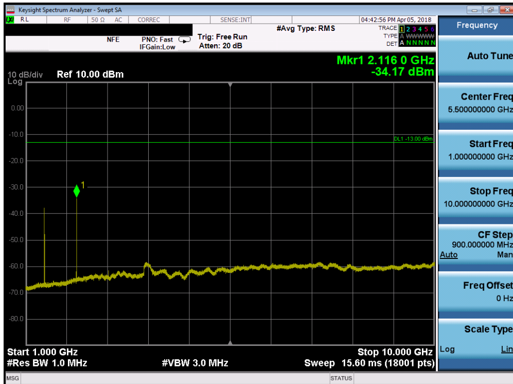
Plot 7-46. Conducted Spurious Plot (Band 12 - 5.0MHz QPSK - RB Size 1, RB Offset 0 - Mid Channel)
