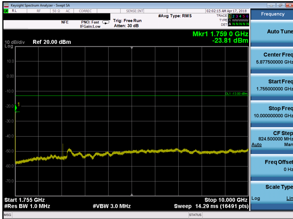
Plot 7-63. Conducted Spurious Plot (Band 4/66 - 10.0MHz QPSK - RB Size 1, RB Offset 0 - Mid Channel)
