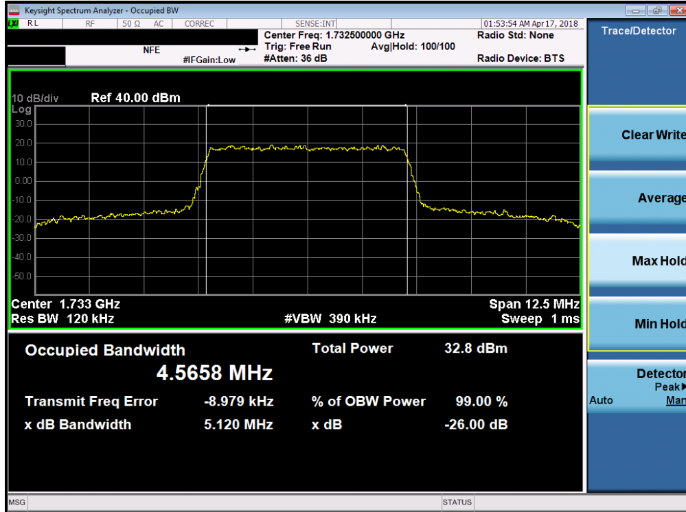
Plot 7-21. Occupied Bandwidth Plot (Band 4/66 - 5.0MHz QPSK - Full RB Configuration)
