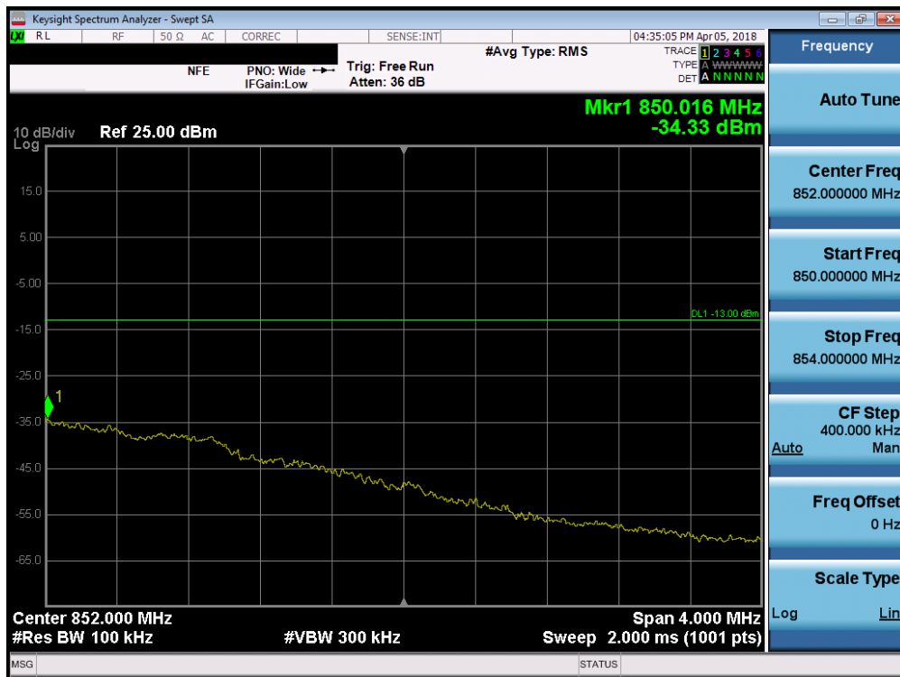
Plot 7-88. Upper Extended Band Edge Plot (Band 5 - 1.4MHz QPSK - Full RB Configuration)
