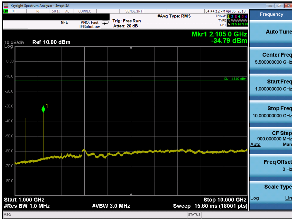
Plot 7-43. Conducted Spurious Plot (Band 12 - 5.0MHz QPSK - RB Size 1, RB Offset 0 - Low Channel)
