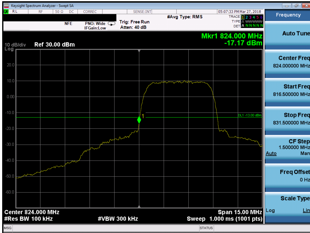
Plot 7-59. Band Edge Plot (Cellular WCDMA Mode - Low Channel)
