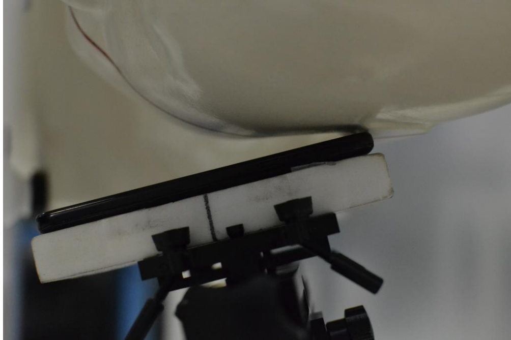
SAR Test Setup Photo 4 – Left Tilt
