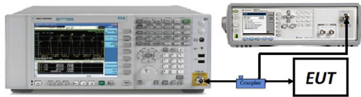
Figure 7-4. Test Instrument & Measurement Setup
