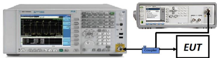
Figure 7-2. Test Instrument & Measurement Setup
