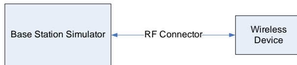
Figure 9-3 Power Measurement Setup
