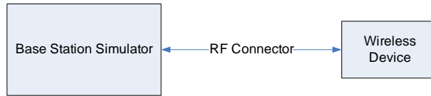
Figure 9-2 Power Measurement Setup
