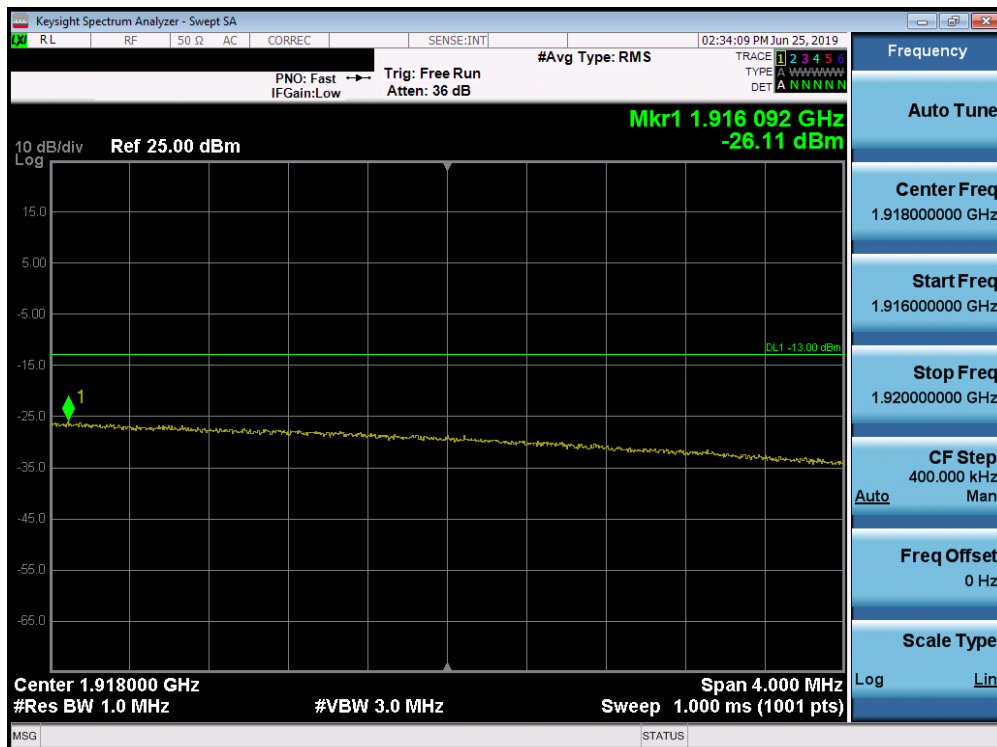
Plot 7-270. Upper Extended Band Edge Plot (Band 25 - 20.0MHz QPSK - Full RB Configuration)
