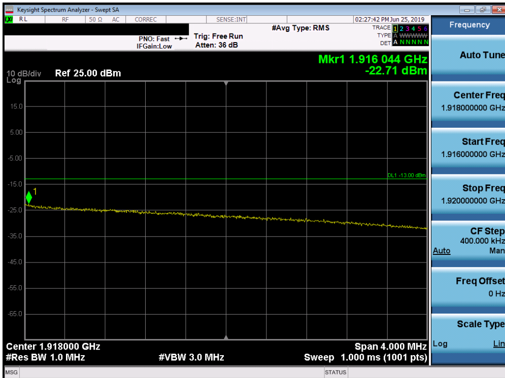
Plot 7-258. Upper Extended Band Edge Plot (Band 25 - 10.0MHz QPSK - Full RB Configuration)
