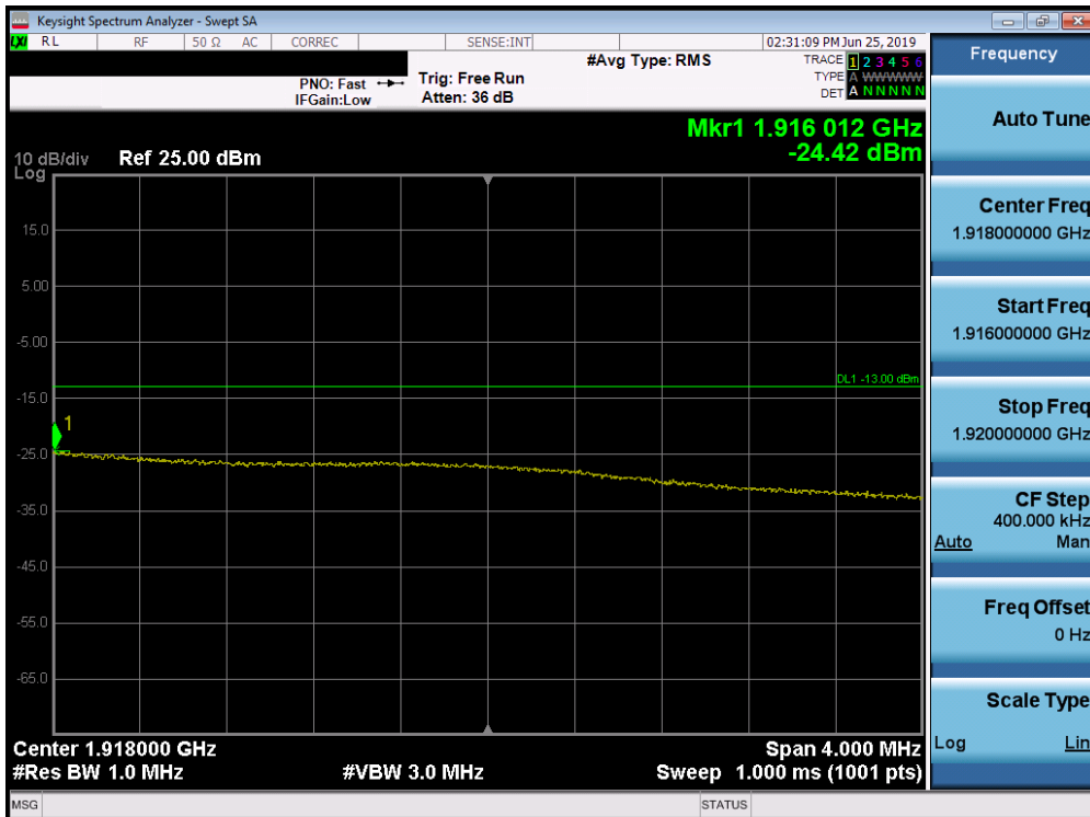
Plot 7-264. Upper Extended Band Edge Plot (Band 25 - 15.0MHz QPSK - Full RB Configuration)
