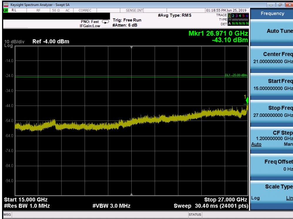
Plot 7-162. Conducted Spurious Plot (Band 41 - 10.0MHz QPSK - RB Size 1, RB Offset 0 - High Channel)
