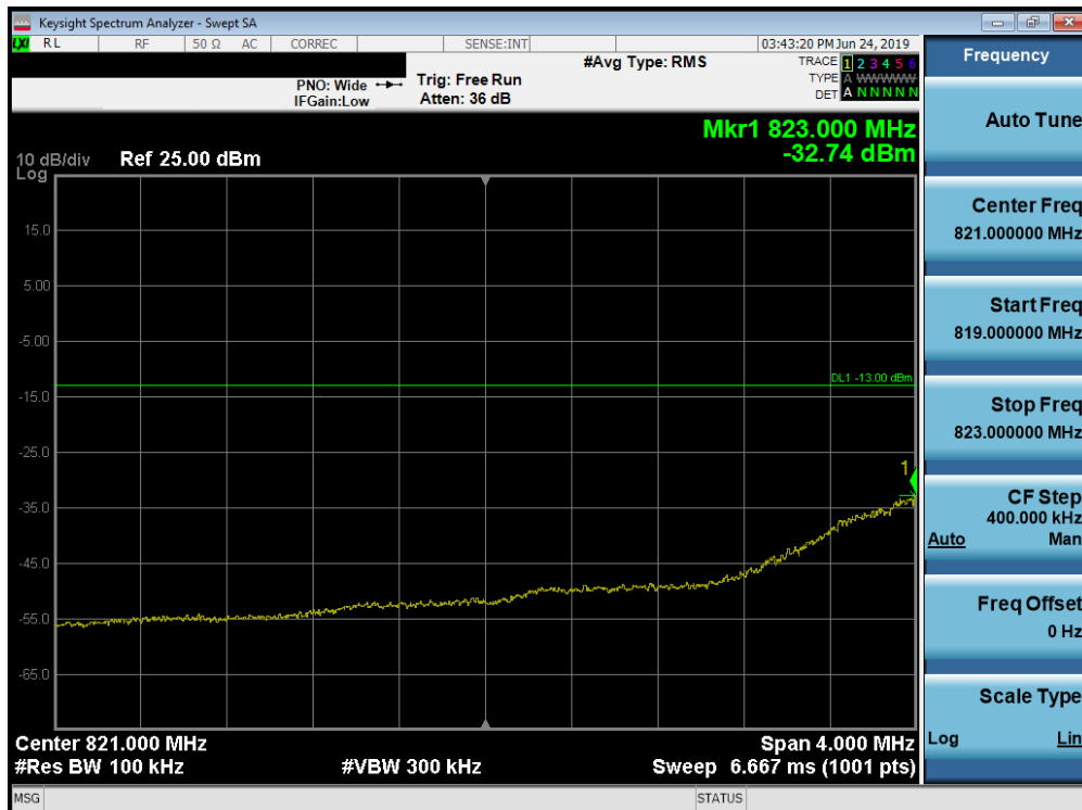
Plot 7-188. Lower Extended Band Edge Plot (Band 26/5 - 1.4MHz QPSK - Full RB Configuration)
