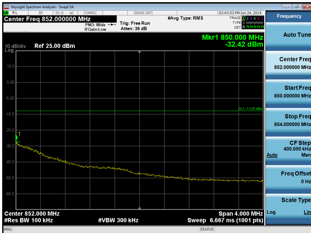
Plot 7-190. Upper Extended Band Edge Plot (Band 26/5 - 1.4MHz QPSK - Full RB Configuration)
