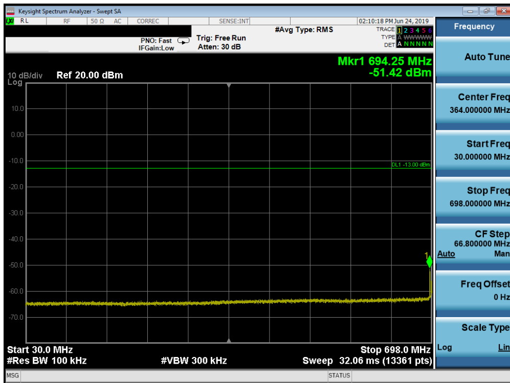
Plot 7-118. Conducted Spurious Plot (Band 12 - 10.0MHz QPSK - RB Size 1, RB Offset 0 - Mid Channel)
