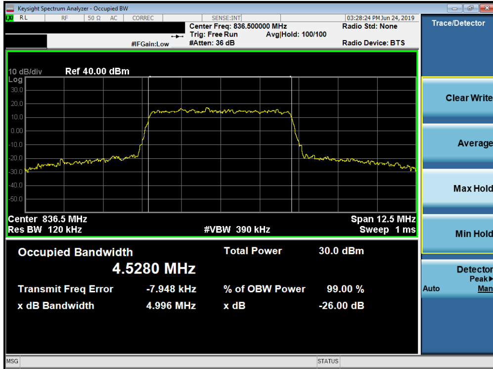
Plot 7-39. Occupied Bandwidth Plot (Band 26/5 - 5.0MHz 64-QAM - Full RB Configuration)
