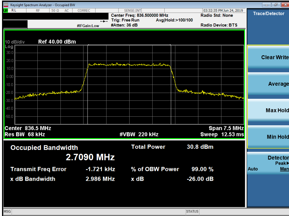
Plot 7-35. Occupied Bandwidth Plot (Band 26/5 - 3.0MHz 16-QAM - Full RB Configuration)
