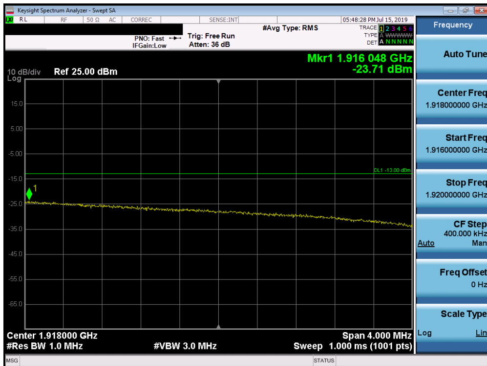
Plot 7-268. Upper Extended Band Edge Plot (Band 25 - 20.0MHz QPSK - Full RB Configuration)
