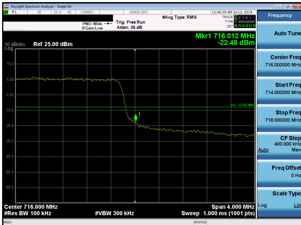
Plot 7-176. Upper Band Edge Plot (Band 12 - 5.0MHz QPSK - Full RB Configuration)
