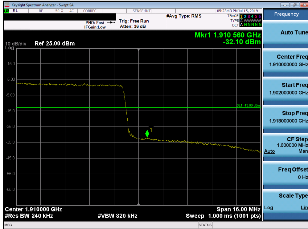
Plot 7-265. Upper Band Edge Plot (Band 2 - 20.0MHz QPSK - Full RB Configuration)
