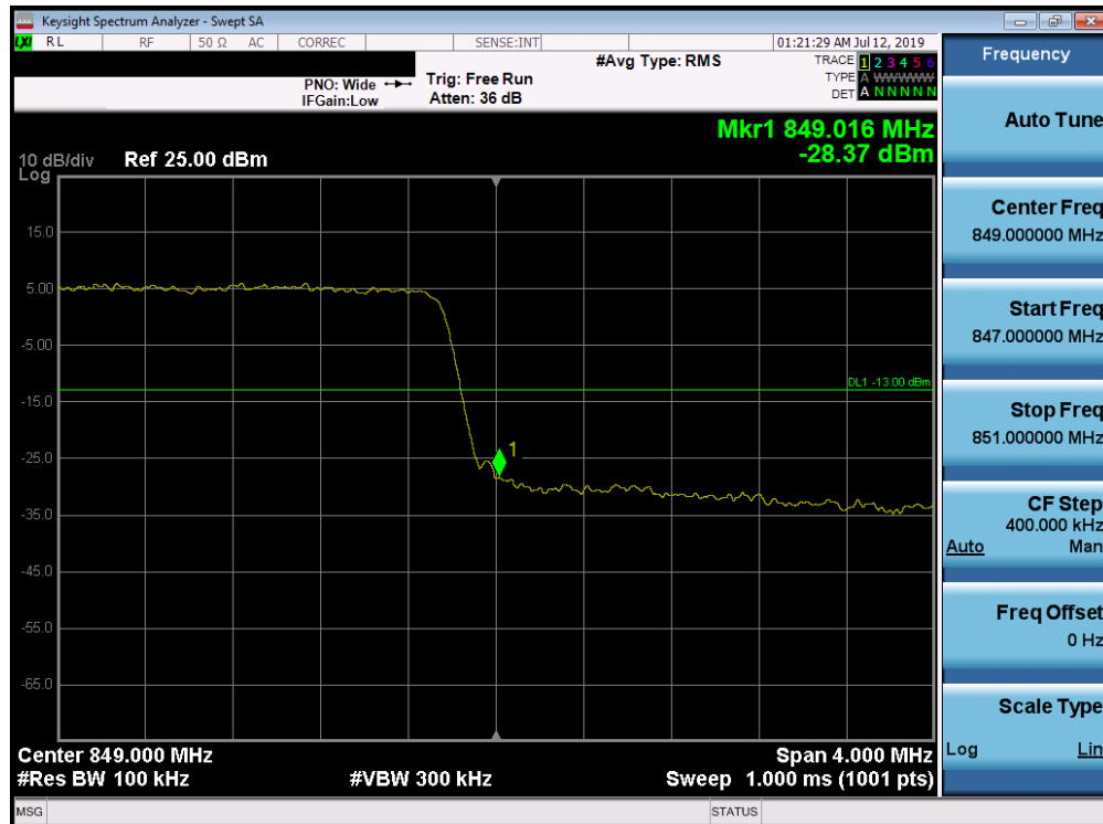
Plot 7-192. Upper Band Edge Plot (Band 26/5 - 5.0MHz QPSK - Full RB Configuration)
