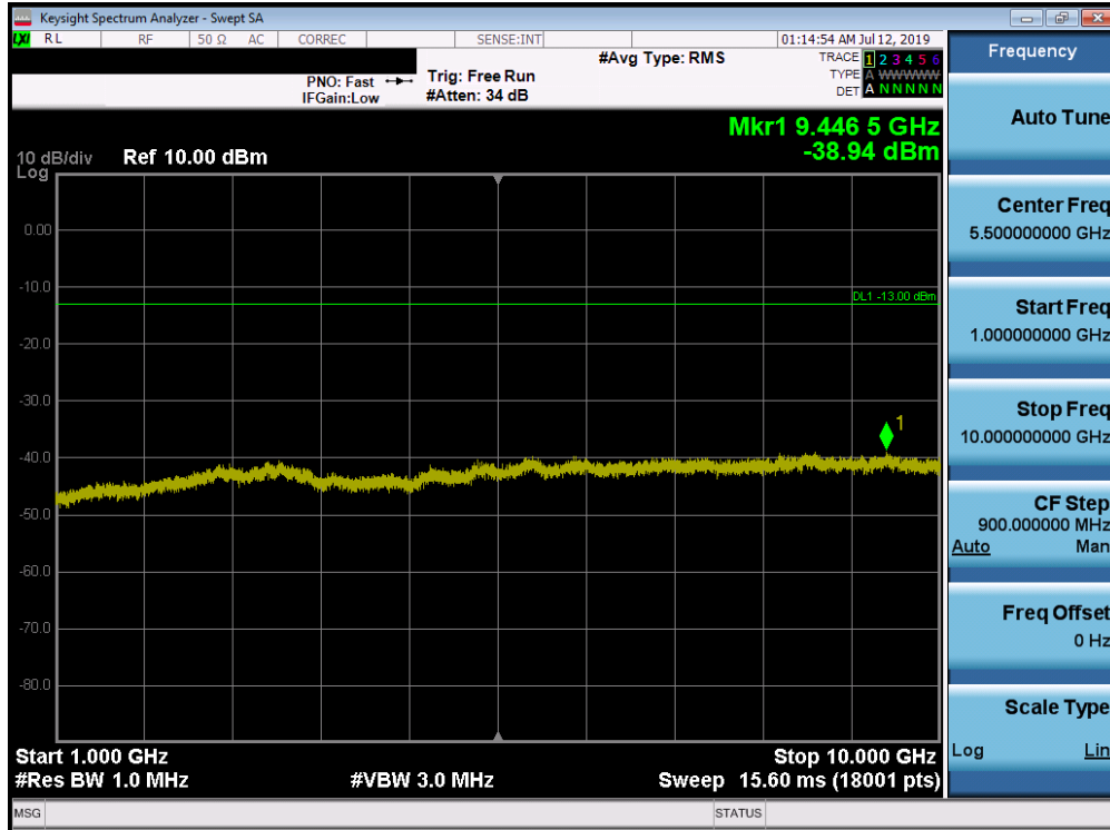
Plot 7-135. Conducted Spurious Plot (Band 26 - 15.0MHz QPSK - RB Size 1, RB Offset 0 - High Channel)
