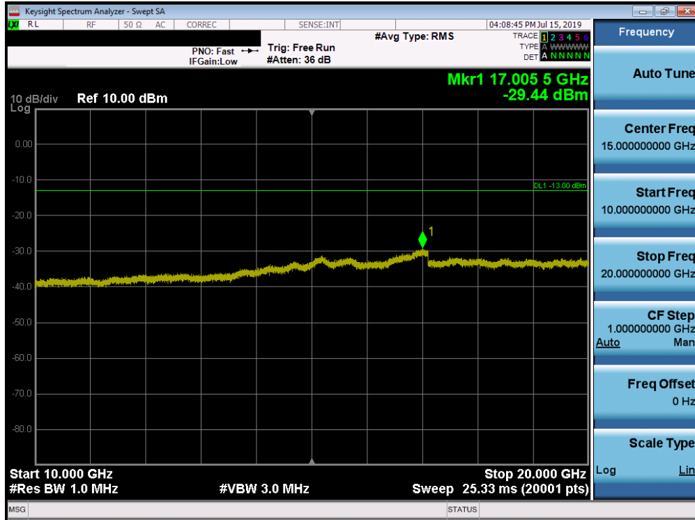
Plot 7-144. Conducted Spurious Plot (Band 66/4 - 20.0MHz QPSK - RB Size 1, RB Offset 0 - High Channel)
