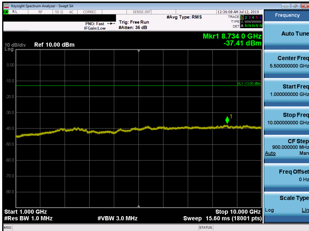
Plot 7-120. Conducted Spurious Plot (Band 12 - 10.0MHz QPSK - RB Size 1, RB Offset 0 - Mid Channel)
