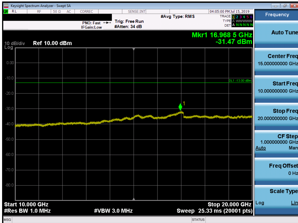
Plot 7-141. Conducted Spurious Plot (Band 66/4 - 20.0MHz QPSK - RB Size 1, RB Offset 0 - Mid Channel)
