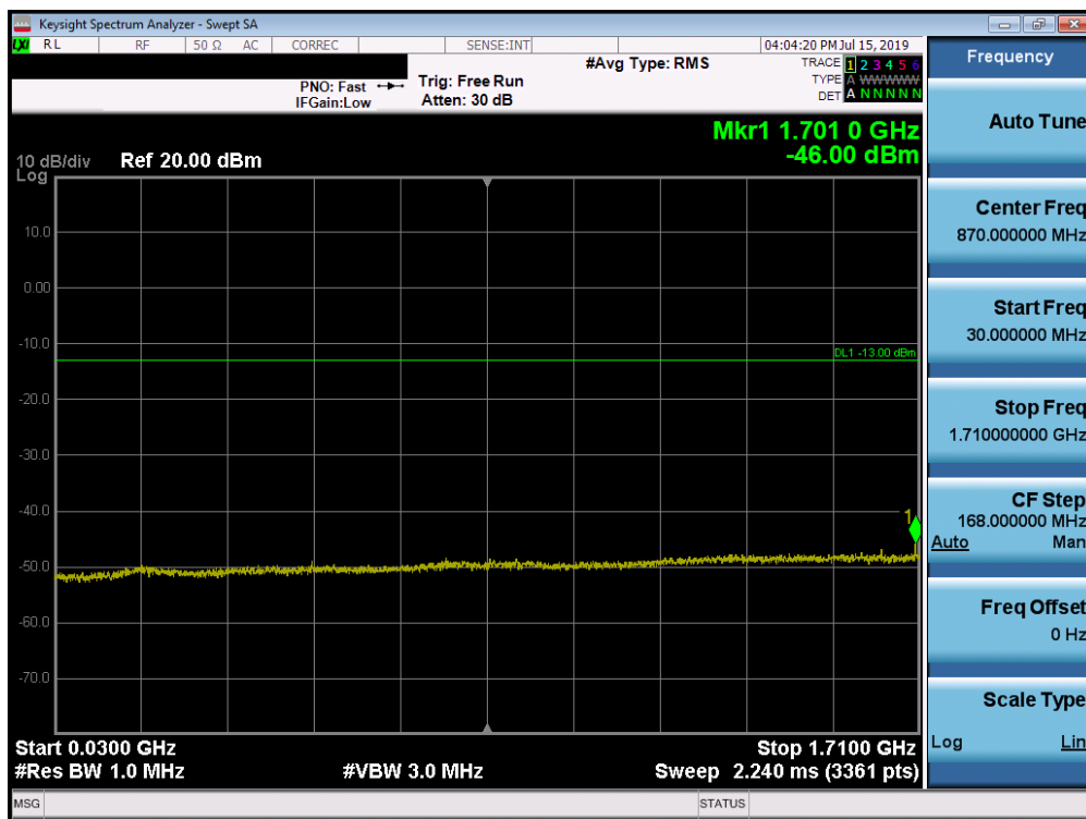
Plot 7-139. Conducted Spurious Plot (Band 66/4 - 20.0MHz QPSK - RB Size 1, RB Offset 0 - Mid Channel)
