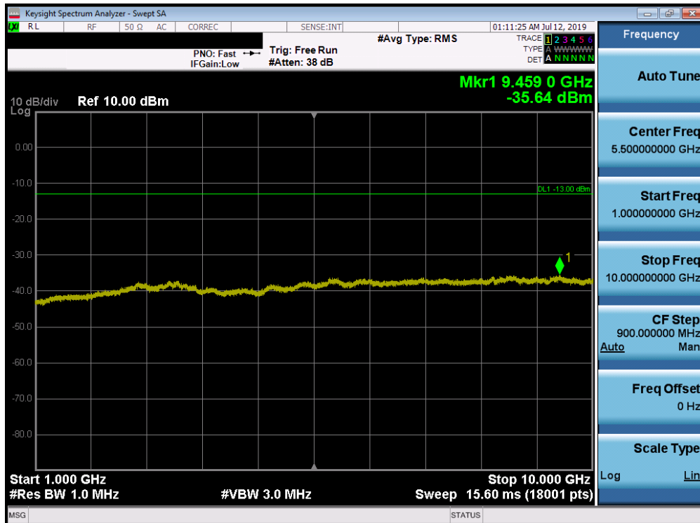
Plot 7-132. Conducted Spurious Plot (Band 26 - 15.0MHz QPSK - RB Size 1, RB Offset 0 - Mid Channel)
