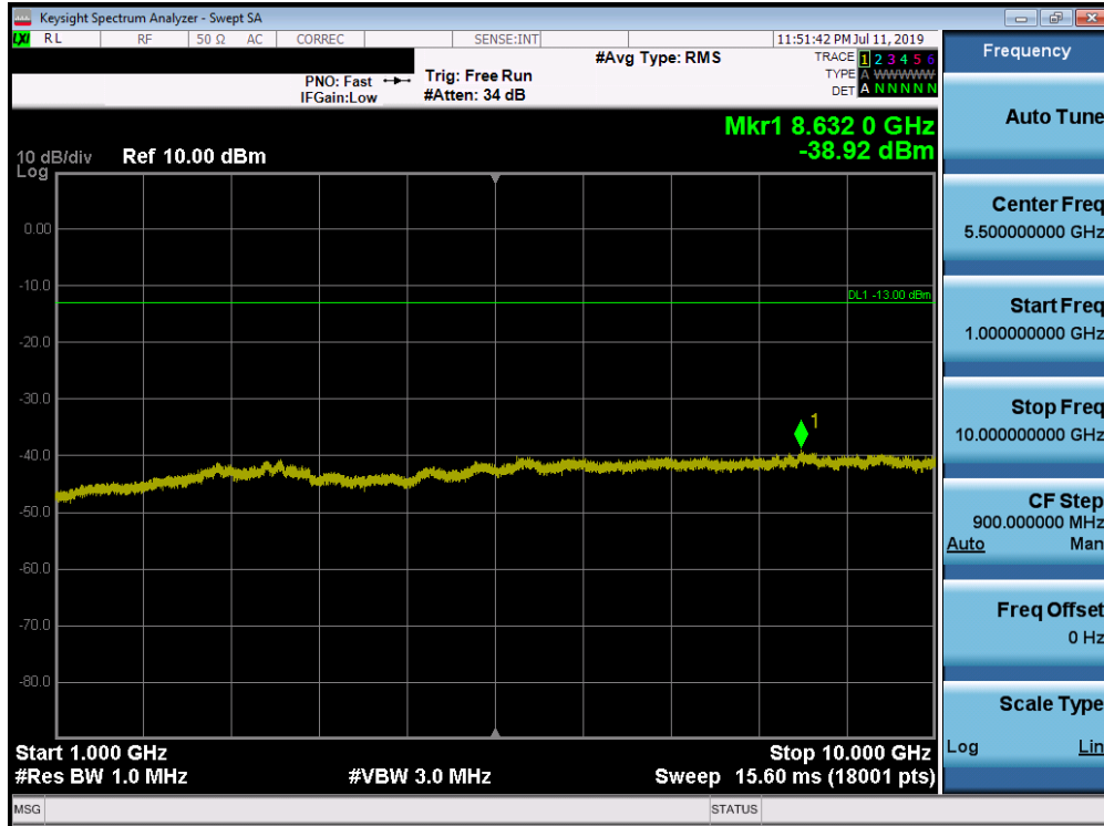
Plot 7-114. Conducted Spurious Plot (Band 71 - 20.0MHz QPSK - RB Size 1, RB Offset 0 - High Channel)
