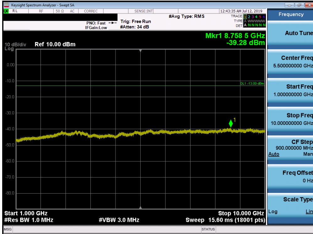
Plot 7-123. Conducted Spurious Plot (Band 12 - 10.0MHz QPSK - RB Size 1, RB Offset 0 - High Channel)
