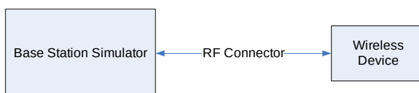
Figure 9-1 Power Measurement Setup
