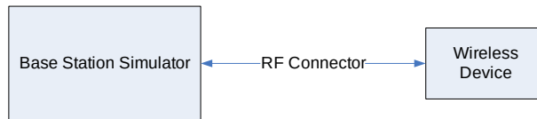
Figure 9-2 Power Measurement Setup
