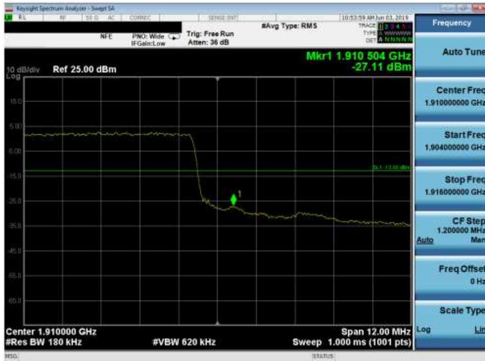
Plot 7-135. Upper Band Edge Plot (Band 2 - 15.0MHz QPSK - Full RB Configuration)
