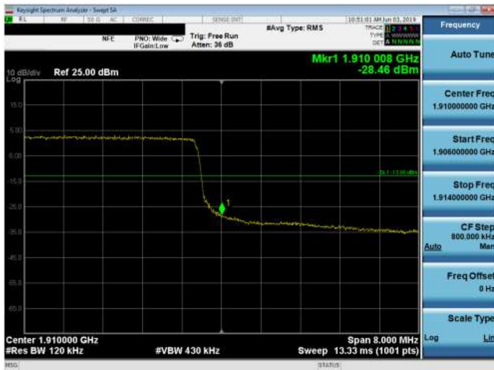
Plot 7-131. Upper Band Edge Plot (Band 2 - 10.0MHz QPSK - Full RB Configuration)
