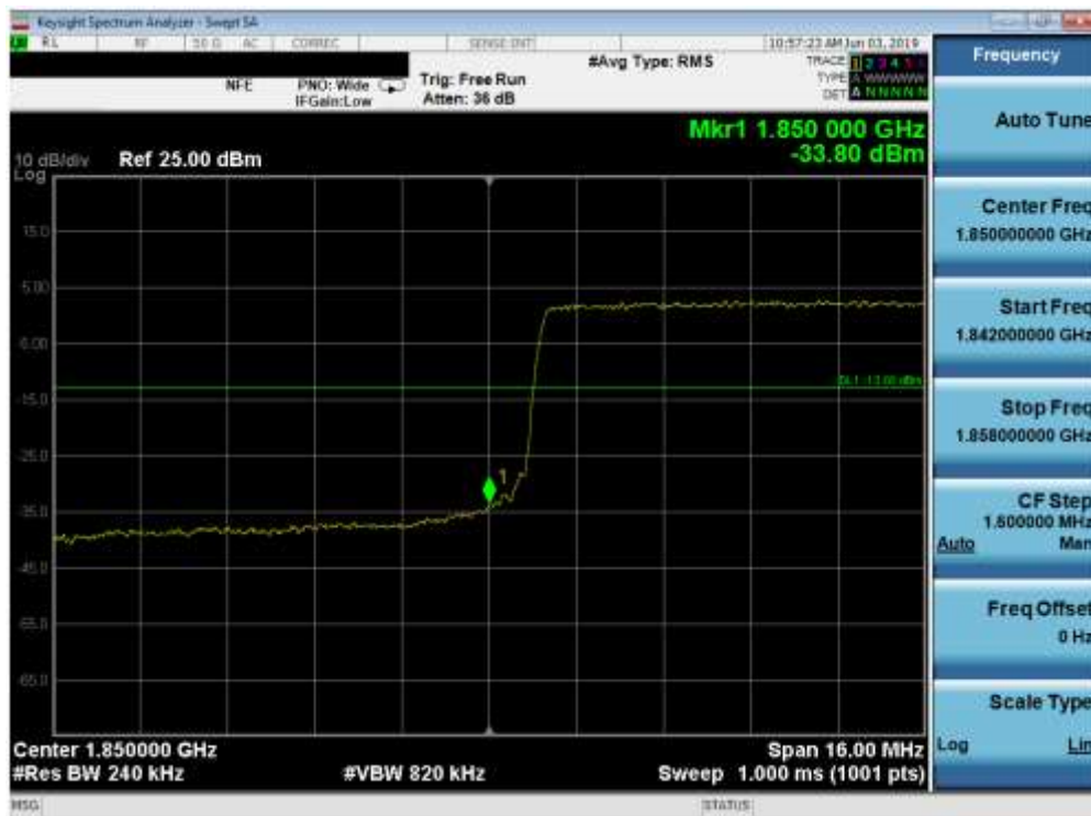
Plot 7-137. Lower Band Edge Plot (Band 2 - 20.0MHz QPSK - Full RB Configuration)
