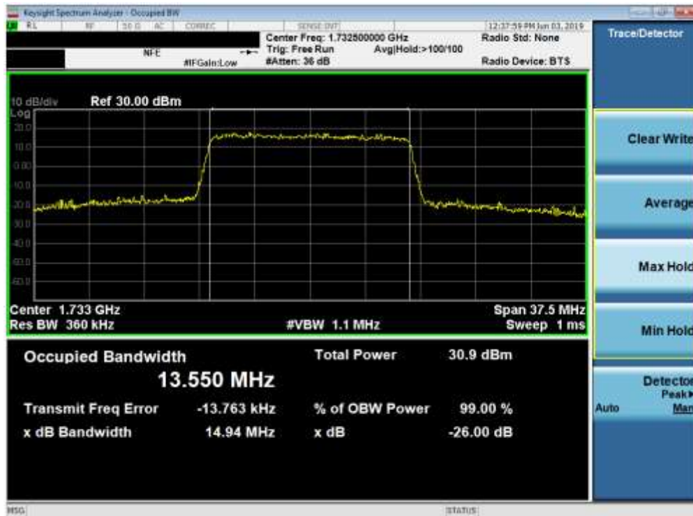
Plot 7-26. Occupied Bandwidth Plot (Band 4 - 15.0MHz 16-QAM - Full RB Configuration)
