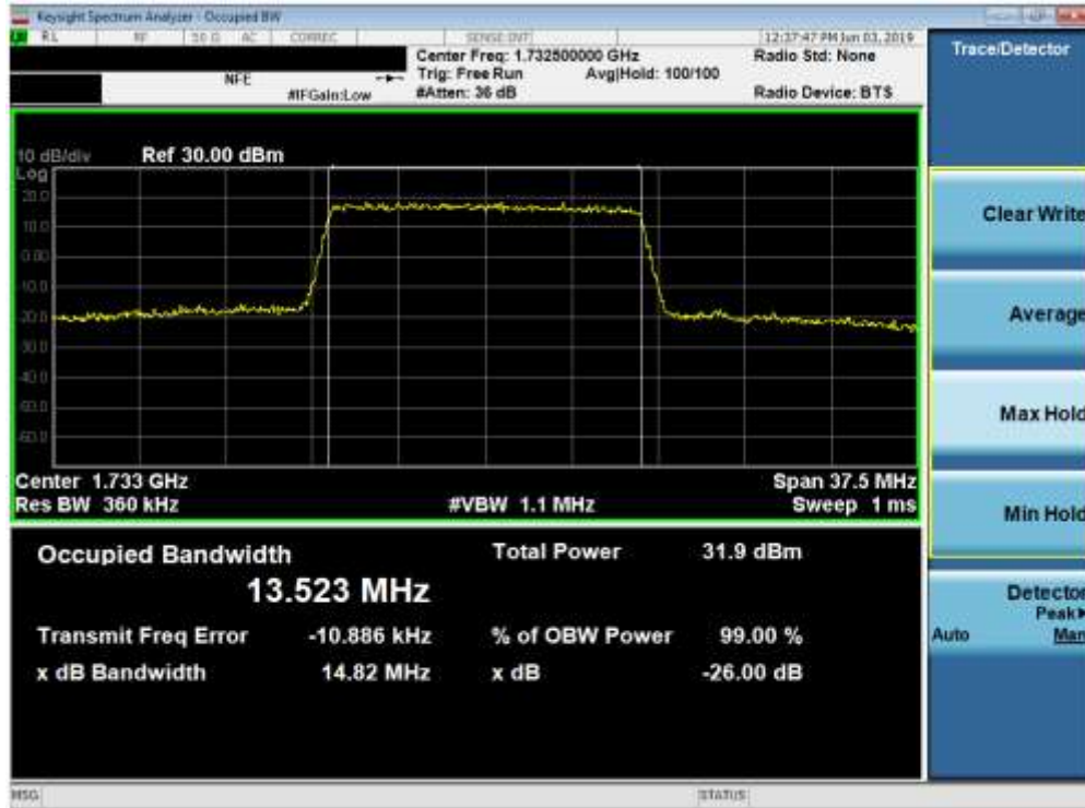
Plot 7-25. Occupied Bandwidth Plot (Band 4 - 15.0MHz QPSK - Full RB Configuration)
