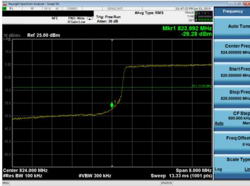
Plot 7-91. Lower Band Edge Plot (Band 5 - 10.0MHz QPSK - Full RB Configuration)
