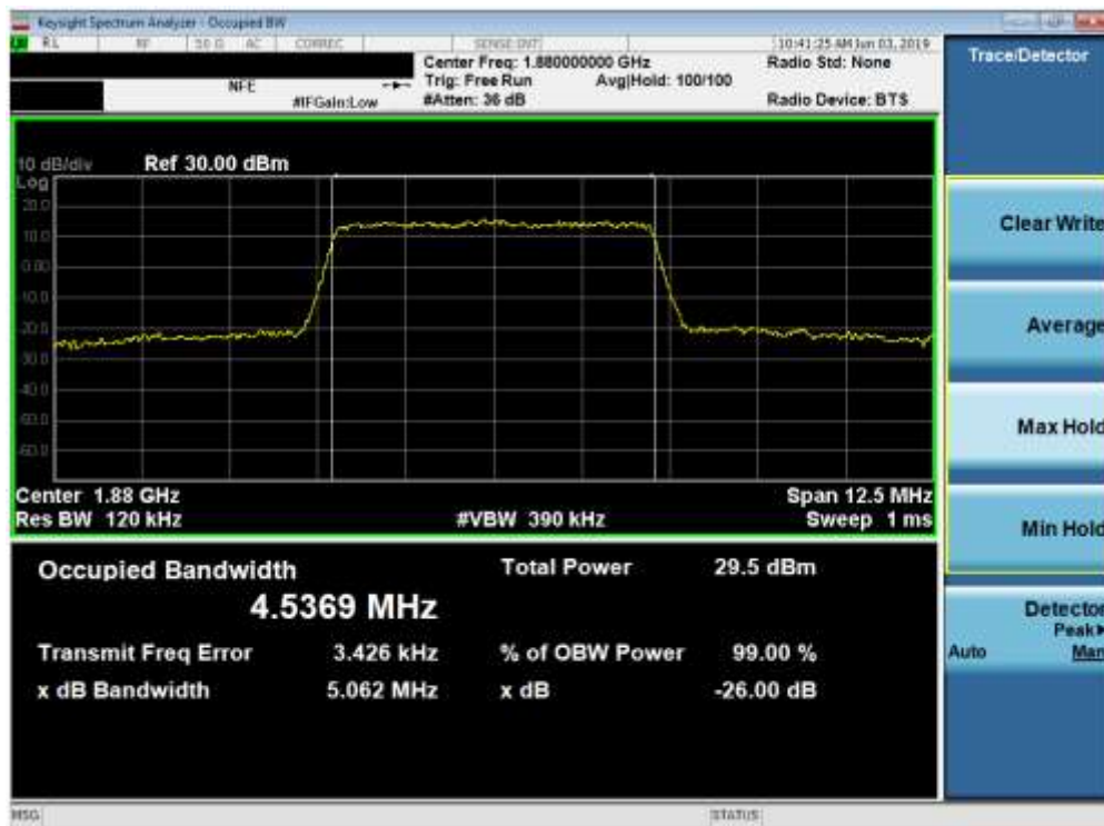
Plot 7-33. Occupied Bandwidth Plot (Band 2 - 5.0MHz QPSK - Full RB Configuration)
