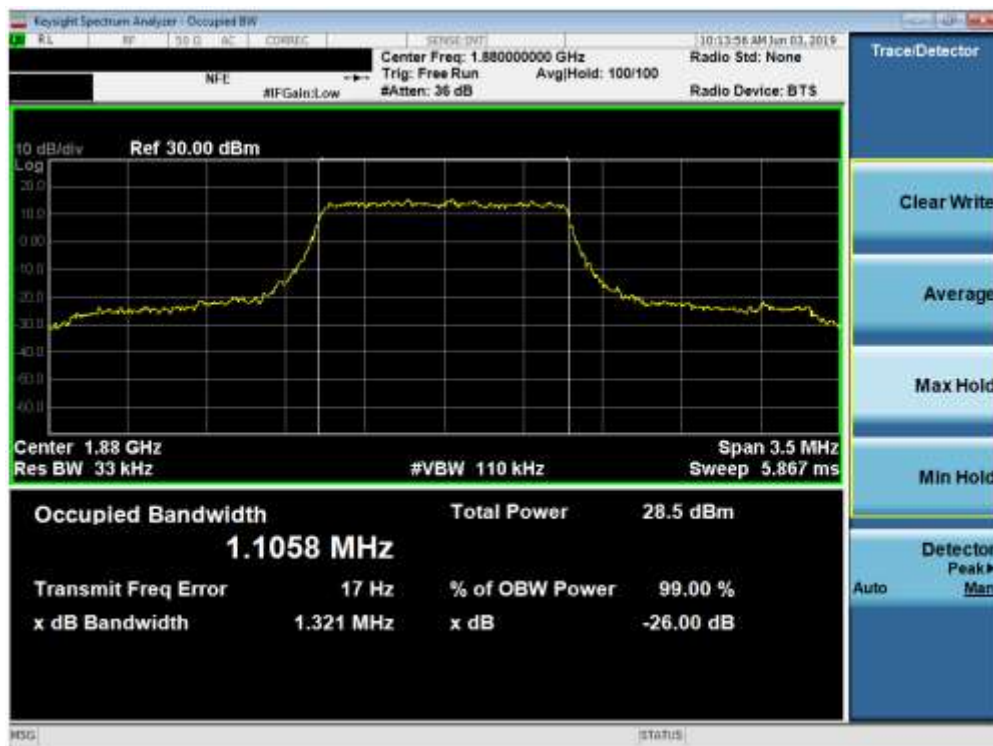
Plot 7-29. Occupied Bandwidth Plot (Band 2 - 1.4MHz QPSK - Full RB Configuration)
