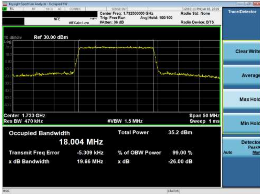
Plot 7-27. Occupied Bandwidth Plot (Band 4 - 20.0MHz QPSK - Full RB Configuration)
