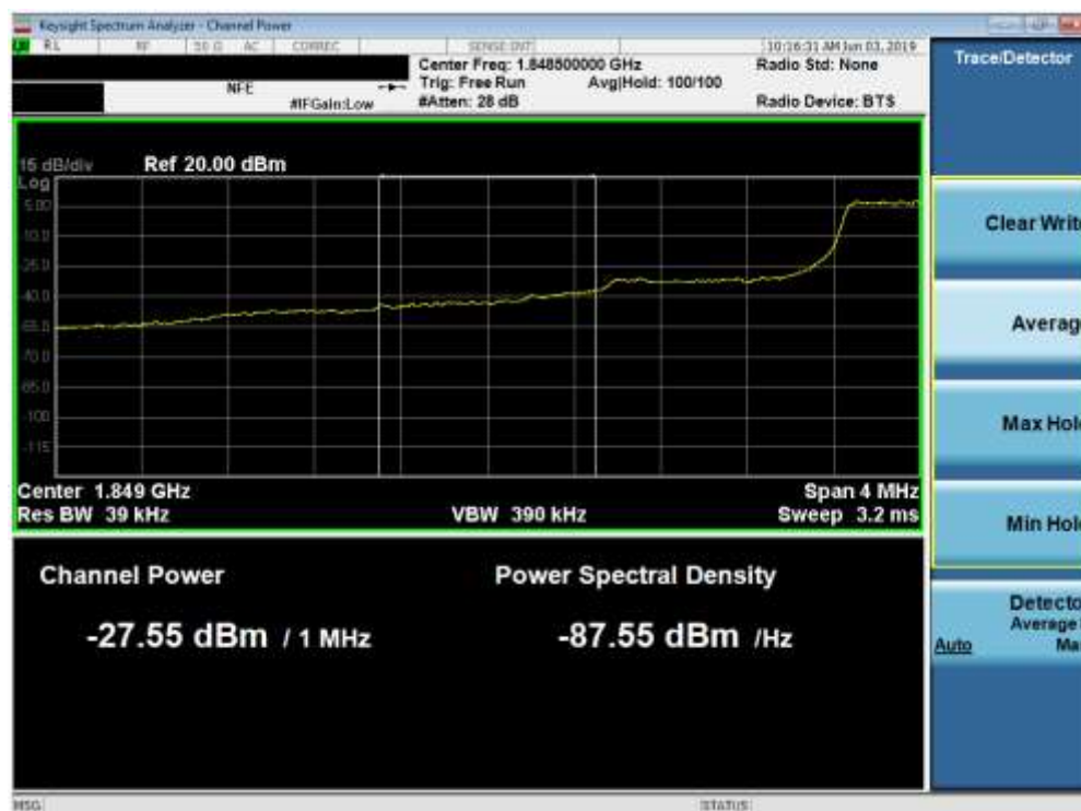
Plot 7-118. Lower Extended Band Edge Plot (Band 2 - 1.4MHz QPSK - Full RB Configuration)
