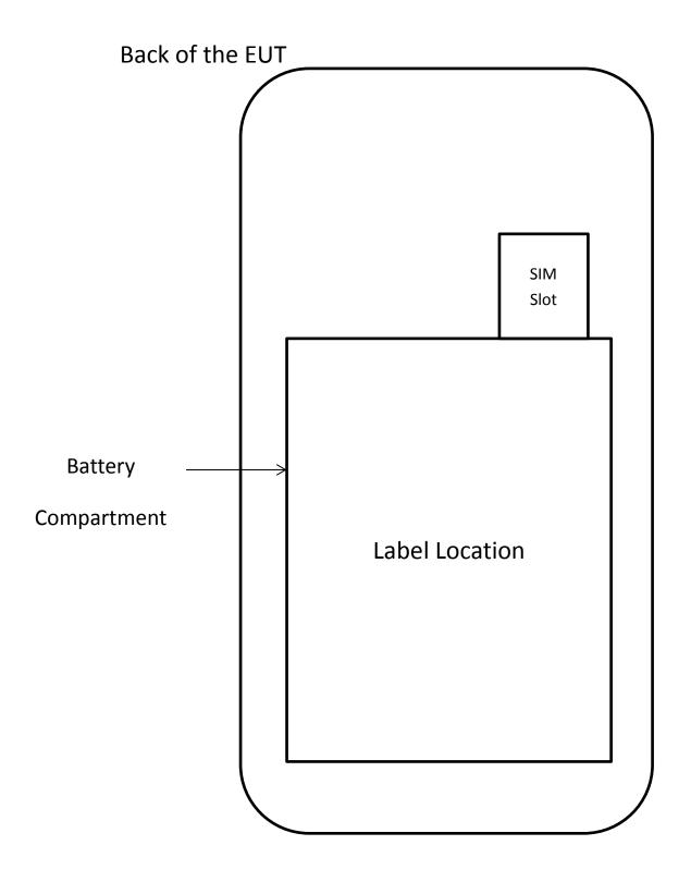
The SIM slot opening is located next to the battery compartment. The end users need to remove the battery firstly in order to install the SIM card, otherwise the SIM card cannot be installed due to physical restrain. The label located in the battery compartment will be visible to the end users when they install the SIM card at the first-time-use.
