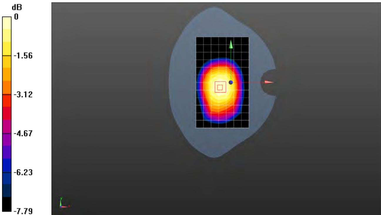
$$0 \text{ dB} = 0.508 \text{ W/kg} = -2.94 \text{ dBW/kg}$$
