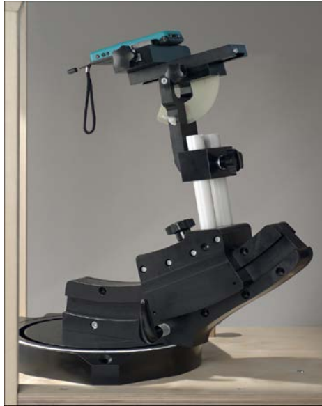
F-2. Device Holder for Transmitters
