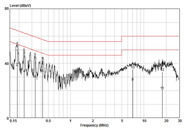
Site : Shielding Room Condition : CE NEUTRAL Job No. : 10750RG Test Mode : BT
