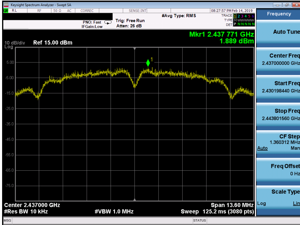
Plot 7-11. Power Spectral Density Plot (802.11b – Ch. 6)
