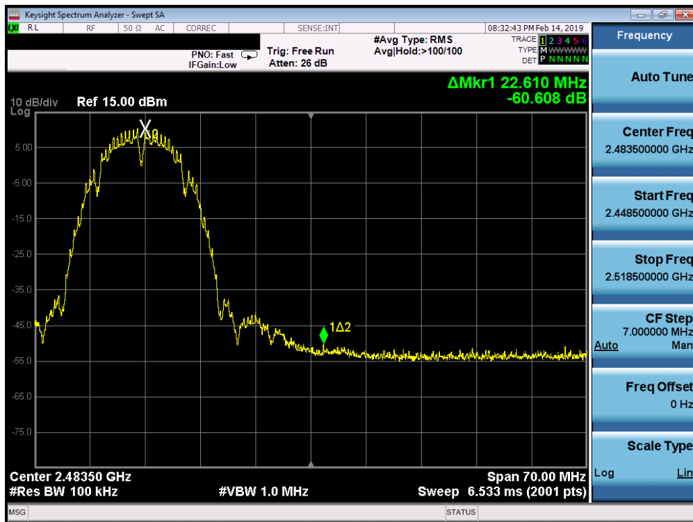
Plot 7-20. Band Edge Plot (802.11b – Ch. 11)
