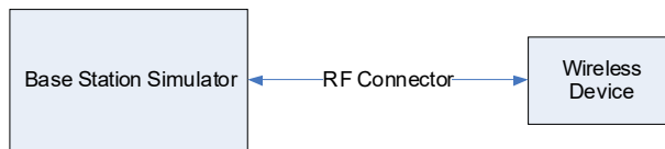
Figure 9-2 Power Measurement Setup
