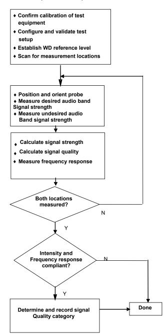
Figure 4-15 C63.19 T-Coil Signal Test Process
