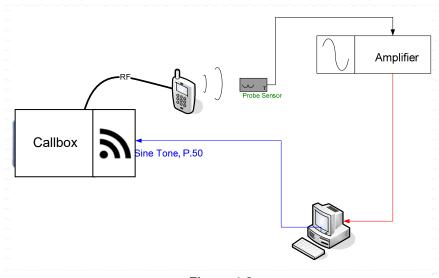
Figure 4-2 T-Coil Test Setup
