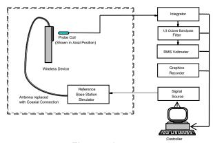
Figure 4-14 **Audio Magnetic Field Test Setup**
