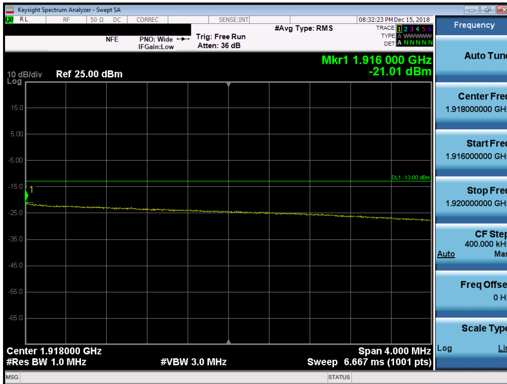
Plot 7-140. Upper Extended Band Edge Plot (Band 25 - 10.0MHz QPSK - Full RB Configuration)
