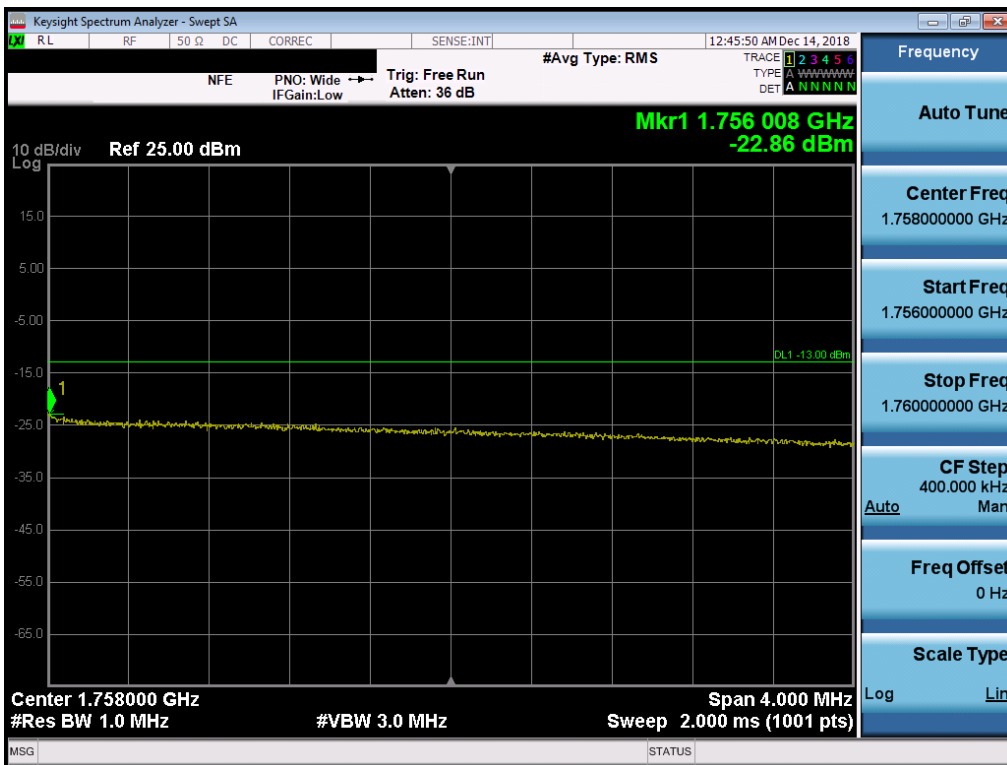
Plot 7-108. Upper Extended Band Edge Plot (Band 4 - 10.0MHz QPSK - Full RB Configuration)
