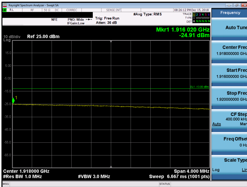
Plot 7-152. Upper Extended Band Edge Plot (Band 25 - 20.0MHz QPSK - Full RB Configuration)
