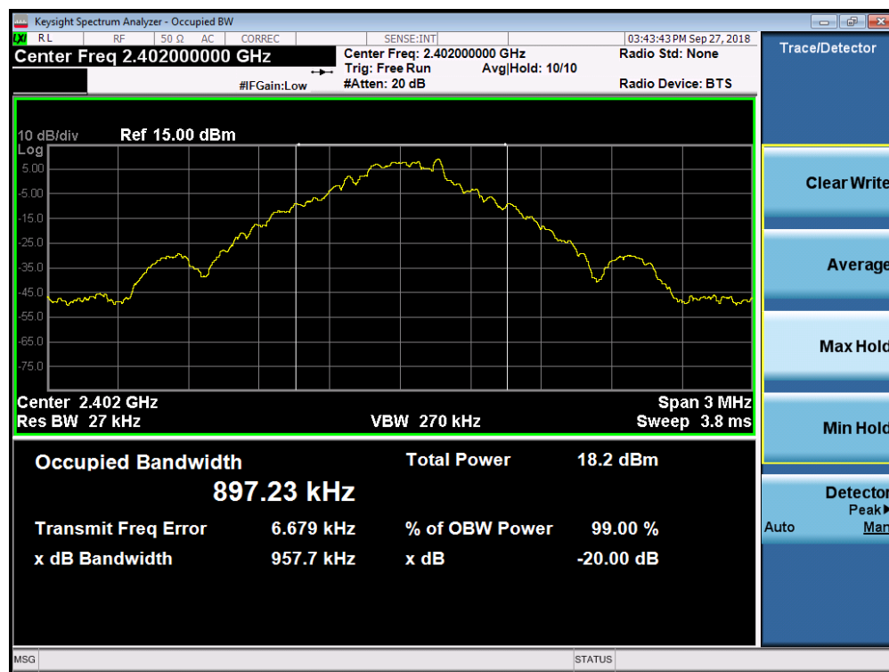
Plot 7-1. 20dB Bandwidth Plot (Bluetooth, 1Mbps – Ch. 0)
