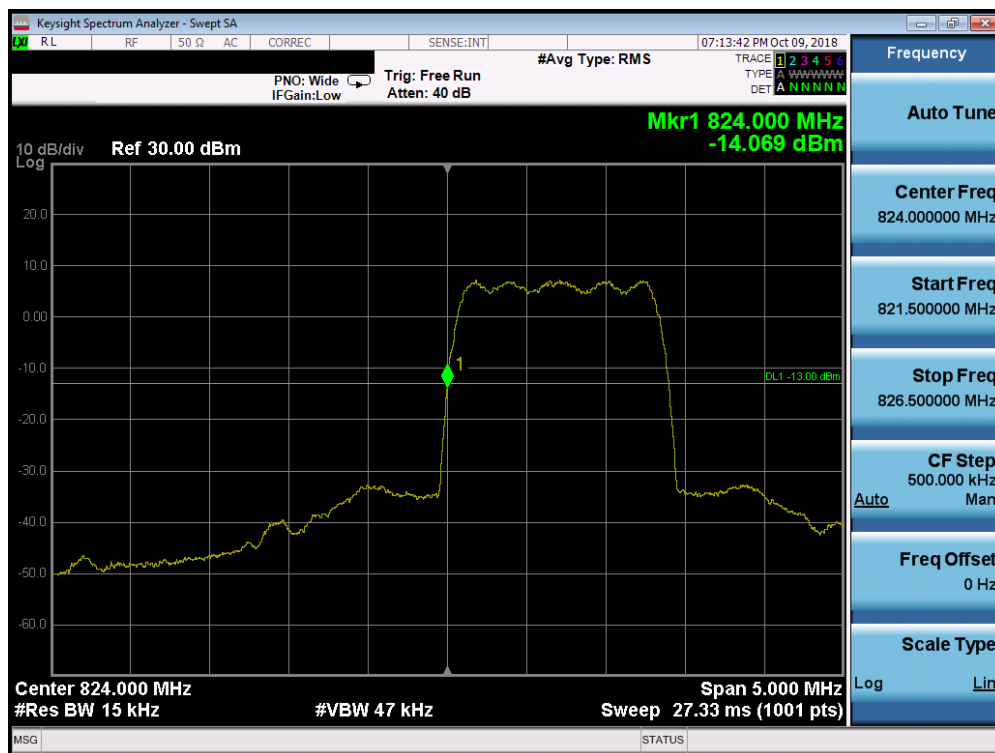
Plot 7-79. Band Edge Plot (Cellular CDMA Mode - Low Channel)
