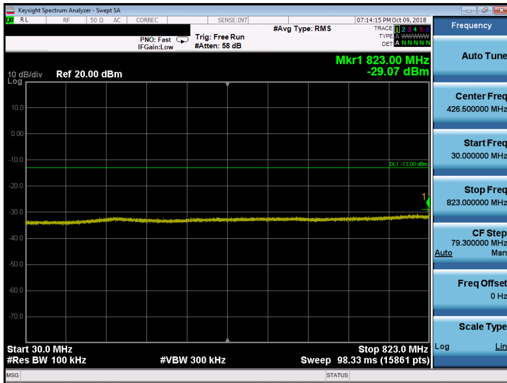
Plot 7-28. Conducted Spurious Plot (Cellular CDMA Mode - Low Channel)
