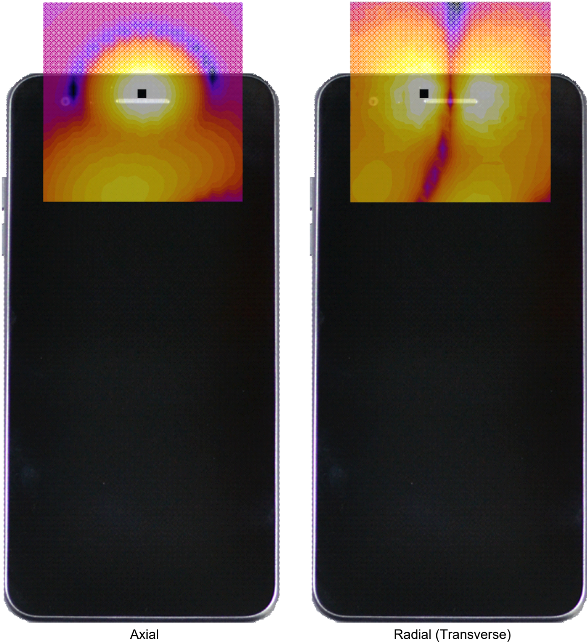
Figure 13-3 T-Coil Scan Overlay Magnetic Field Distributions
