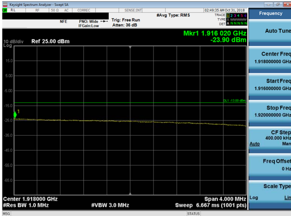
Plot 7-78. Upper Extended Band Edge Plot (Band 25 - 20.0MHz QPSK - Full RB Configuration)
