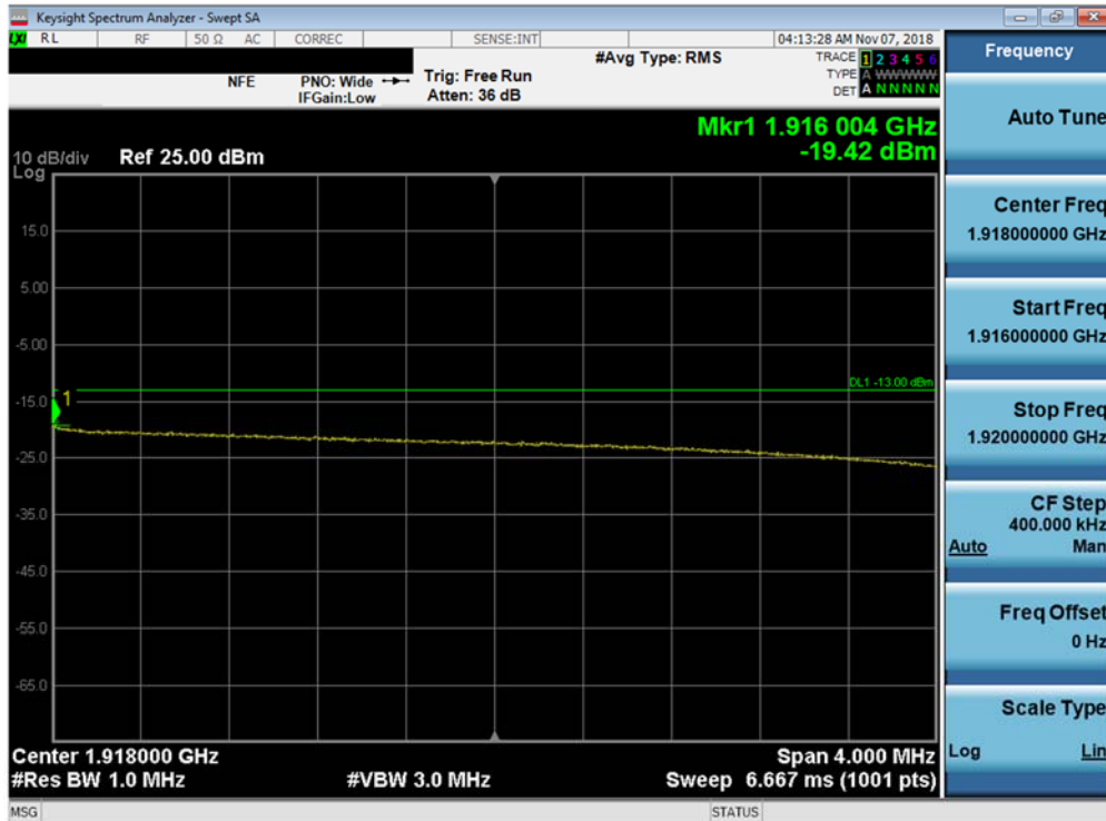
Plot 7-70. Upper Extended Band Edge Plot (Band 25 - 10.0MHz QPSK - Full RB Configuration)
