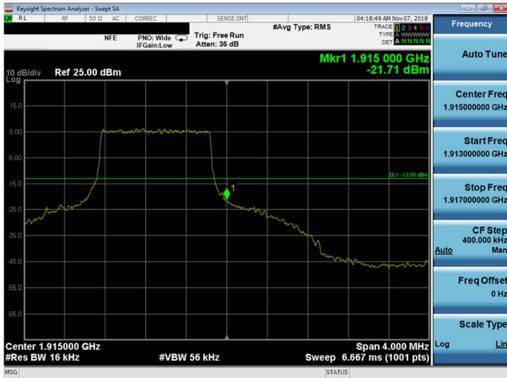
Plot 7-57. Upper Band Edge Plot (Band 25 - 1.4MHz QPSK - Full RB Configuration)
