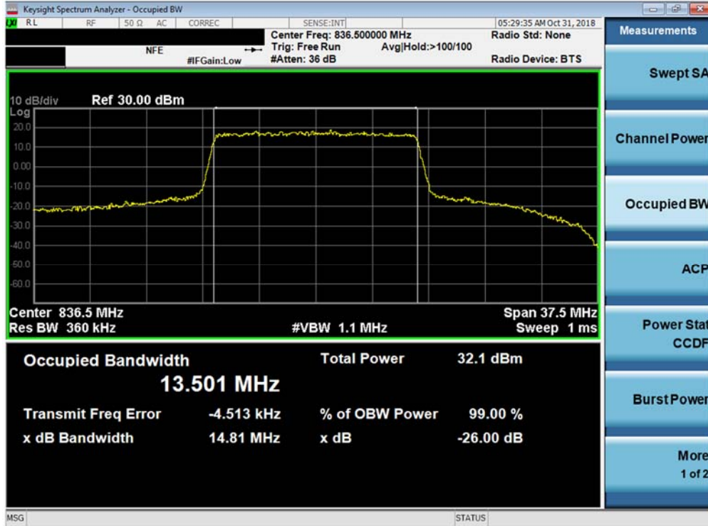
Plot 7-9. Occupied Bandwidth Plot (Band 26 - 15.0MHz QPSK - Full RB Configuration)
