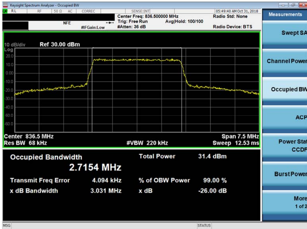
Plot 7-3. Occupied Bandwidth Plot (Band 26 - 3.0MHz QPSK - Full RB Configuration)
