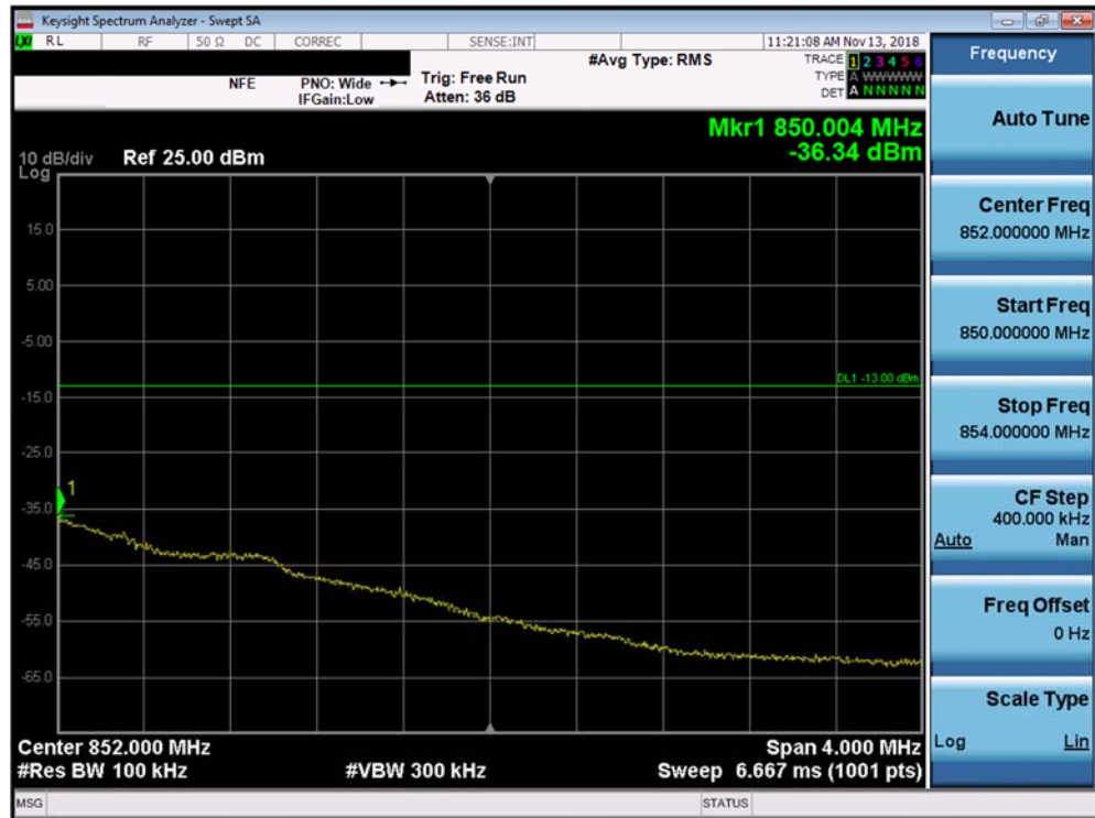
Plot 7-44. Upper Extended Band Band Edge Plot (Band 26 - 1.4MHz QPSK - Full RB Configuration)
