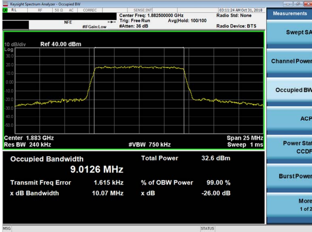
Plot 7-17. Occupied Bandwidth Plot (Band 25 - 10.0MHz QPSK - Full RB Configuration)
