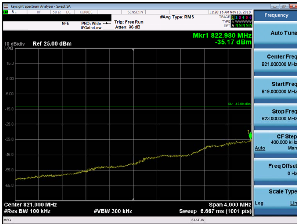
Plot 7-42. Lower Extended Band Edge Plot (Band 26 - 1.4MHz QPSK - Full RB Configuration)
