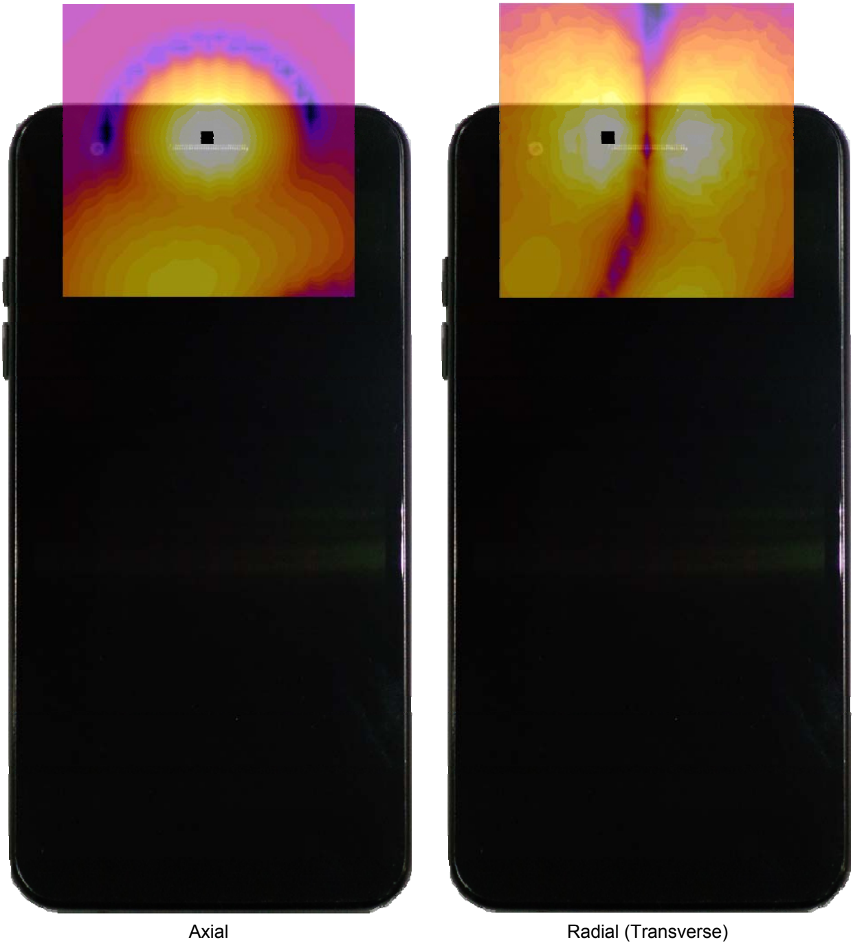
Figure 16-3 T-Coil Scan Overlay Magnetic Field Distributions
