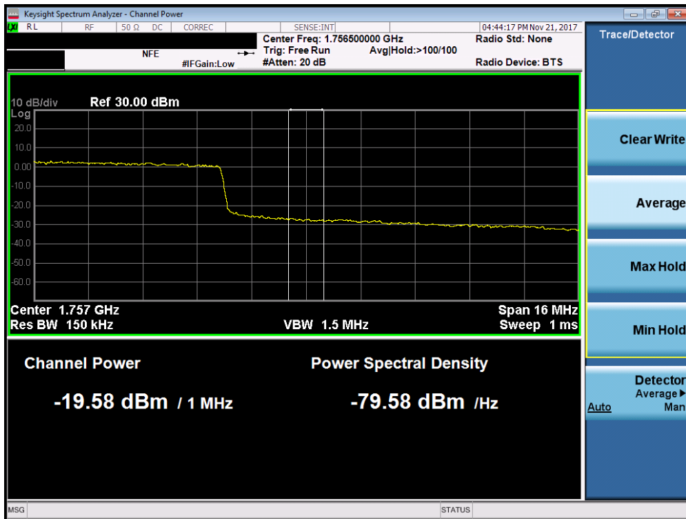
Plot 7-112. Upper Extended Band Edge Plot (Band 4 - 20.0MHz QPSK - Full RB Configuration)
