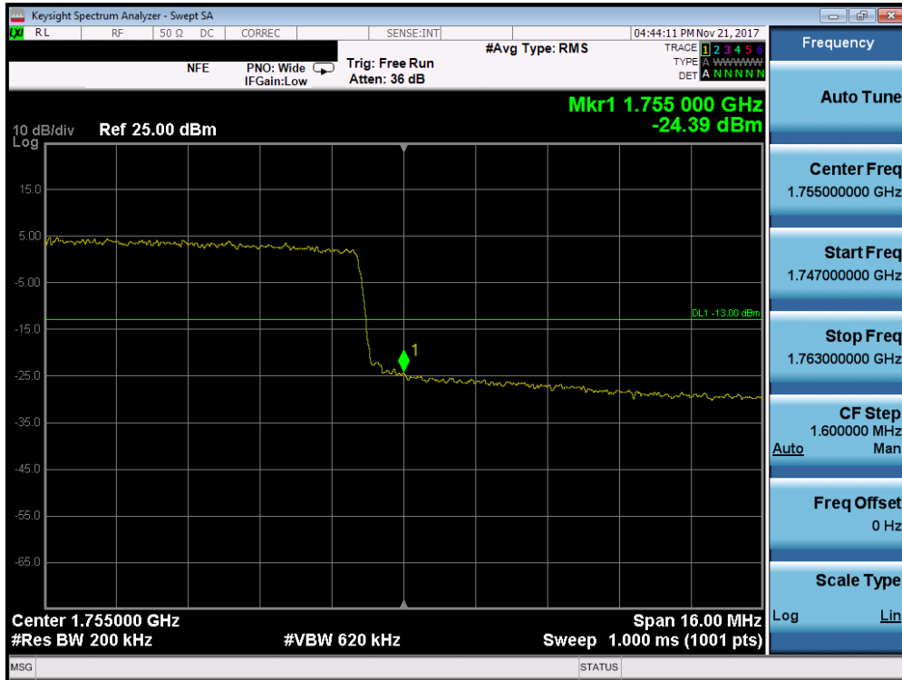
Plot 7-111. Upper Band Edge Plot (Band 4 - 20.0MHz QPSK - Full RB Configuration)
