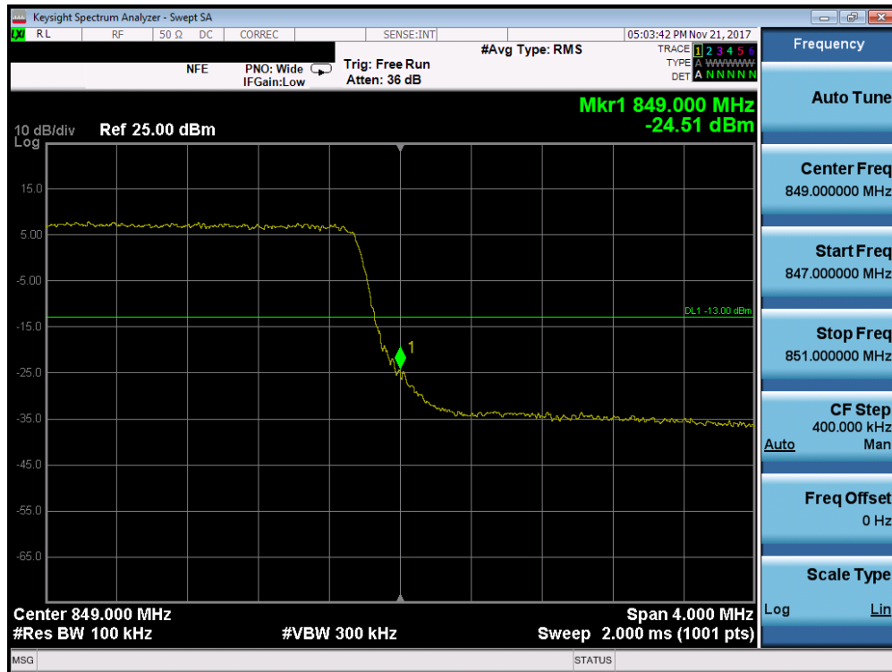
Plot 7-86. Upper Band Edge Plot (Band 5 - 5.0MHz QPSK - Full RB Configuration)
