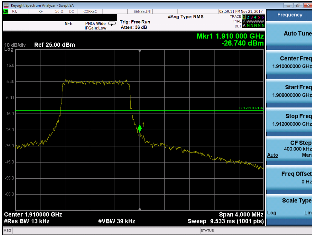
Plot 7-115. Upper Band Edge Plot (Band 2 - 1.4MHz QPSK - Full RB Configuration)
