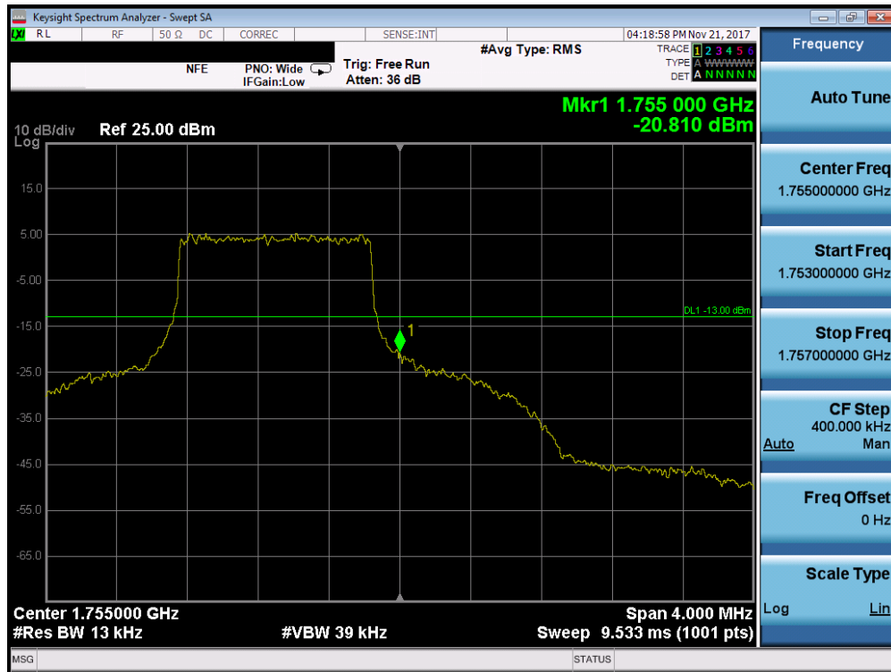
Plot 7-91. Upper Band Edge Plot (Band 4 - 1.4MHz QPSK - Full RB Configuration)
