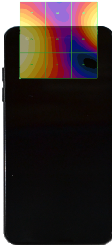
Figure 17-4 E-Field WD Scan overlay
