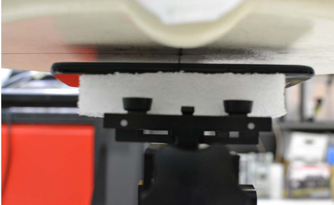
SAR Test Setup Photo 5: Back side at 1.0 cm
