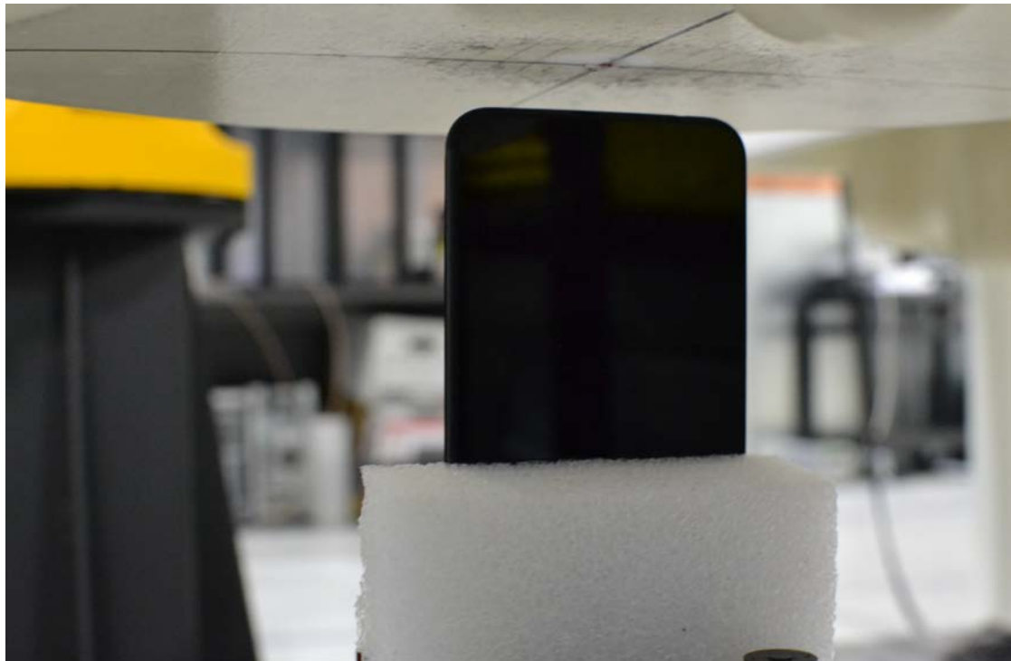
SAR Test Setup Photo 8: Bottom Edge at 1.0 cm
