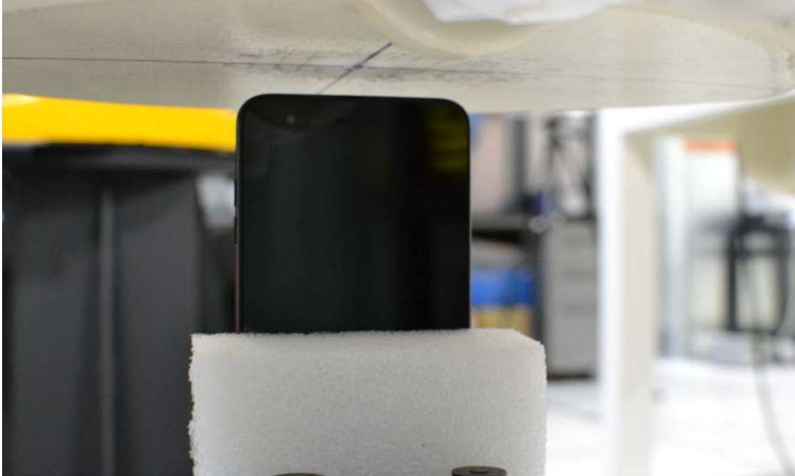
SAR Test Setup Photo 7: Top Edge at 1.0 cm
