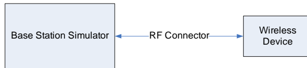
Figure 9-1 Power Measurement Setup
