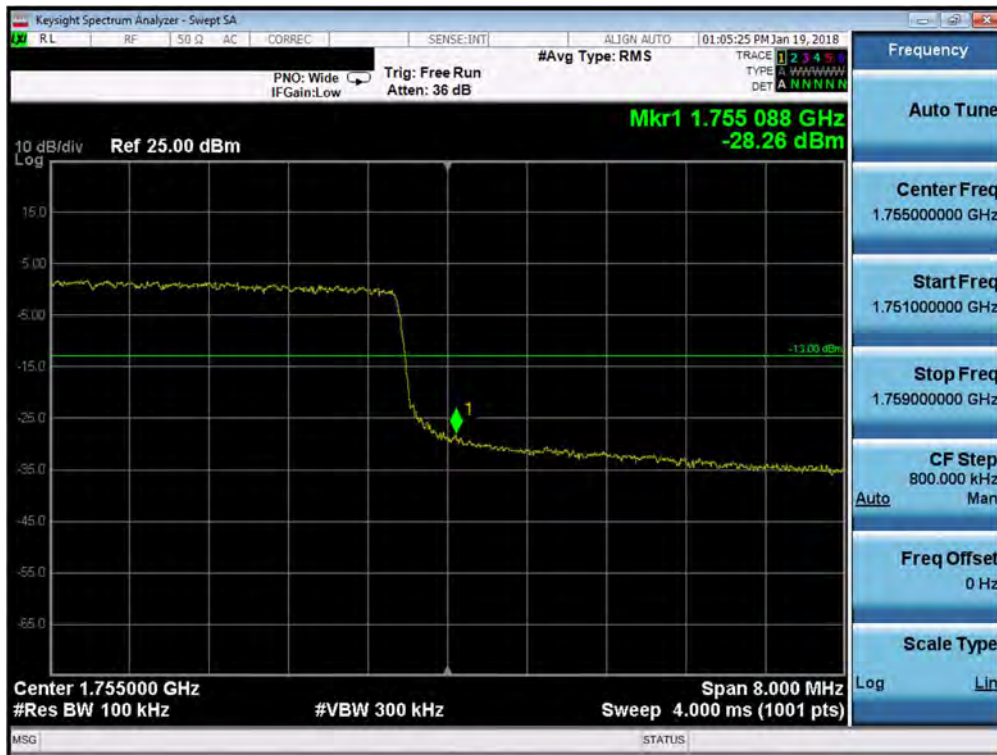
Plot 7-107. Lower Extended Band Edge Plot (Band 4 - 10.0MHz QPSK - Full RB Configuration)
