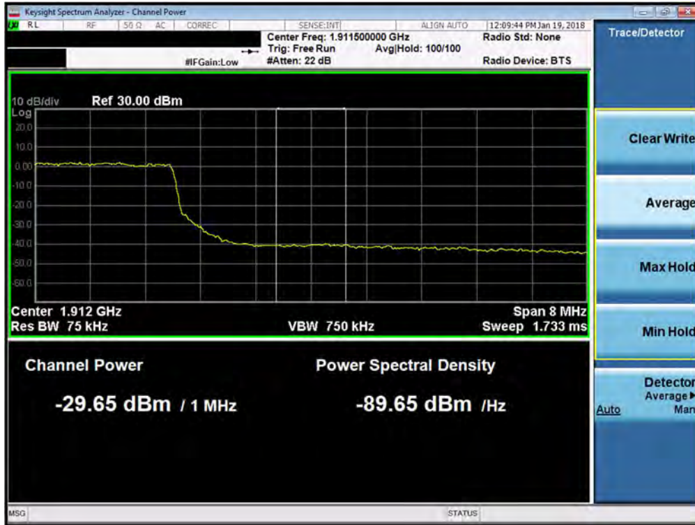
Plot 7-140. Upper Extended Band Edge Plot (Band 2 - 10.0MHz QPSK - Full RB Configuration)
