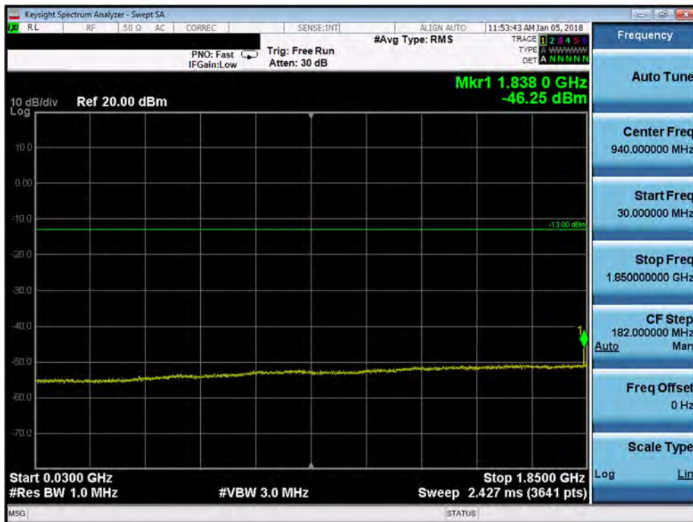
Plot 7-71. Conducted Spurious Plot (Band 2/25 - 20.0MHz QPSK - RB Size 1, RB Offset 0 - Mid Channel)
