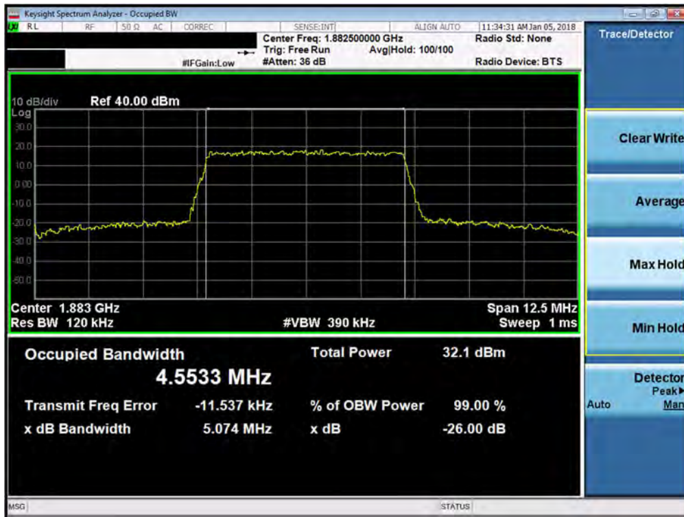
Plot 7-33. Occupied Bandwidth Plot (Band 2/25 - 5.0MHz QPSK - Full RB Configuration)
