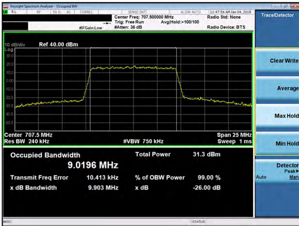
Plot 7-8. Occupied Bandwidth Plot (Band 12 - 10.0MHz 16-QAM - Full RB Configuration)
