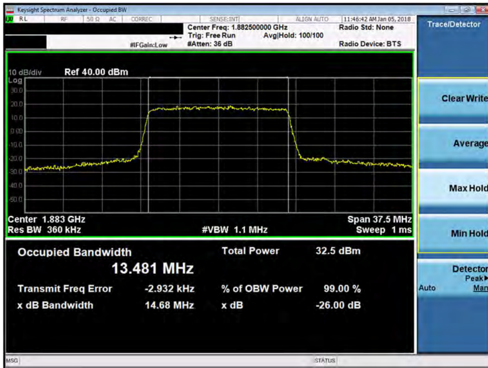
Plot 7-37. Occupied Bandwidth Plot (Band 2/25 - 15.0MHz QPSK - Full RB Configuration)
