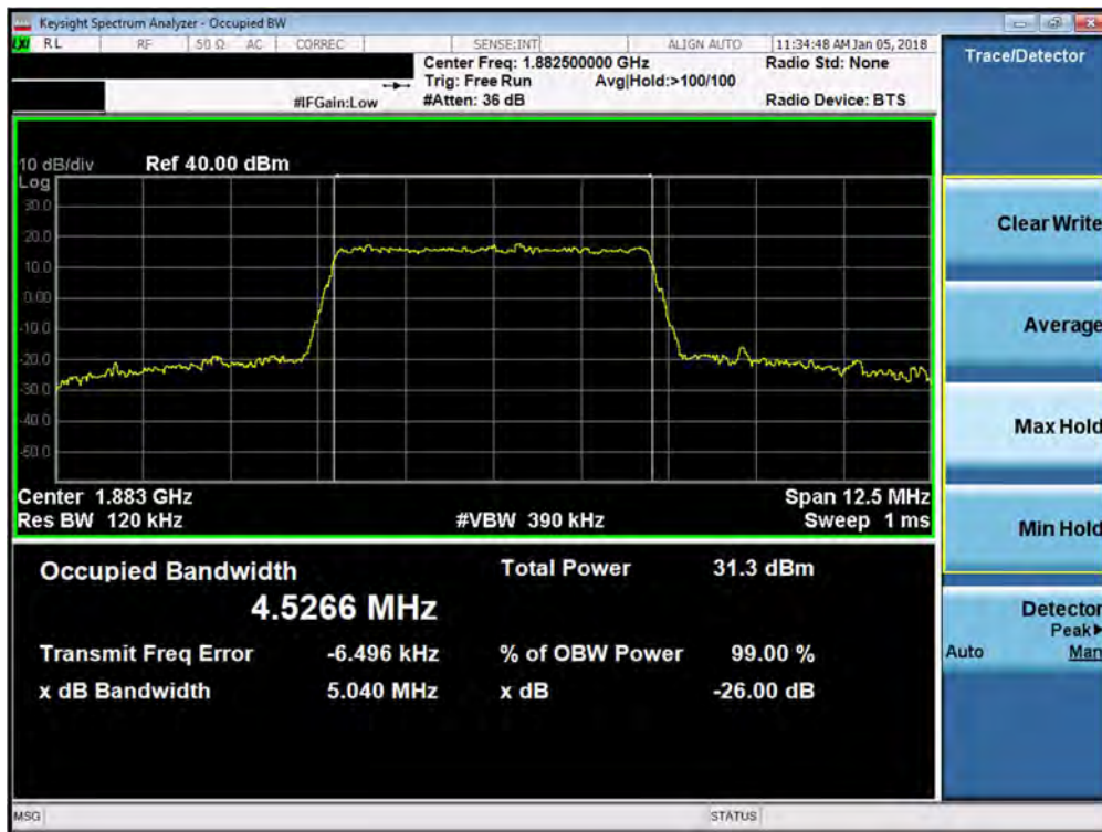
Plot 7-34. Occupied Bandwidth Plot (Band 2/25 - 5.0MHz 16-QAM - Full RB Configuration)
