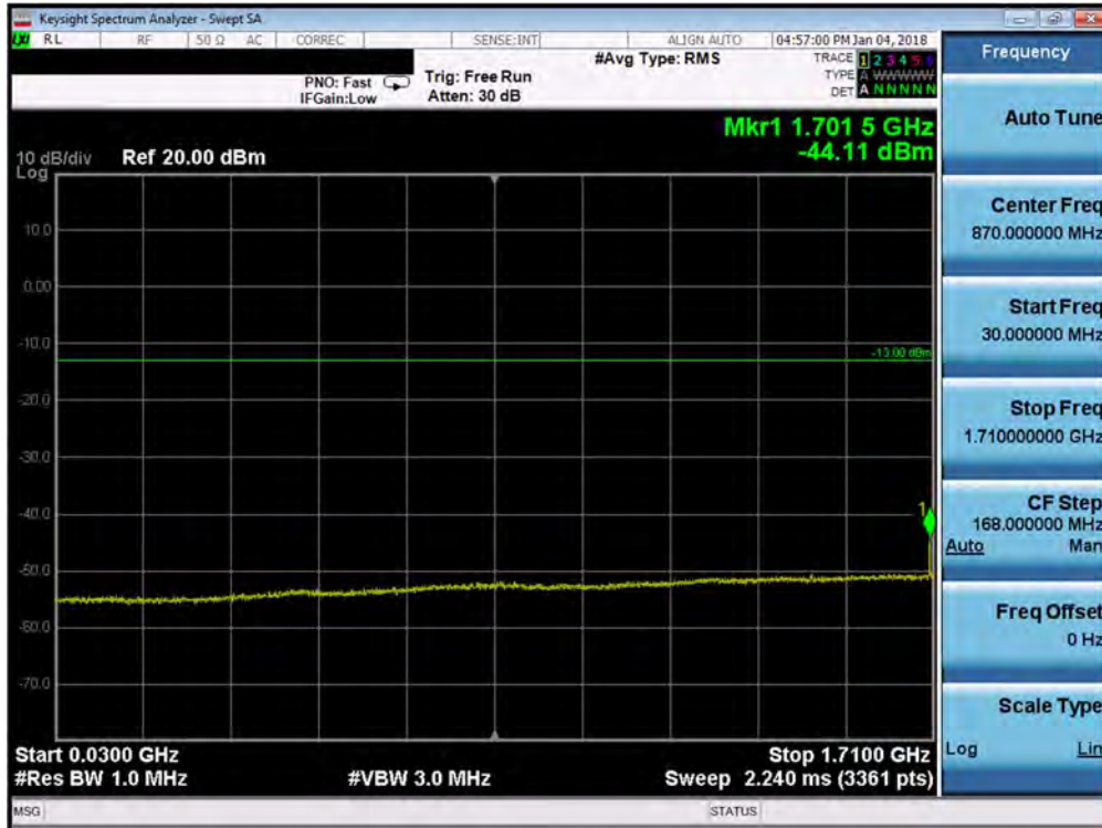
Plot 7-65. Conducted Spurious Plot (Band 4 - 20.0MHz QPSK - RB Size 1, RB Offset 0 - High Channel)
