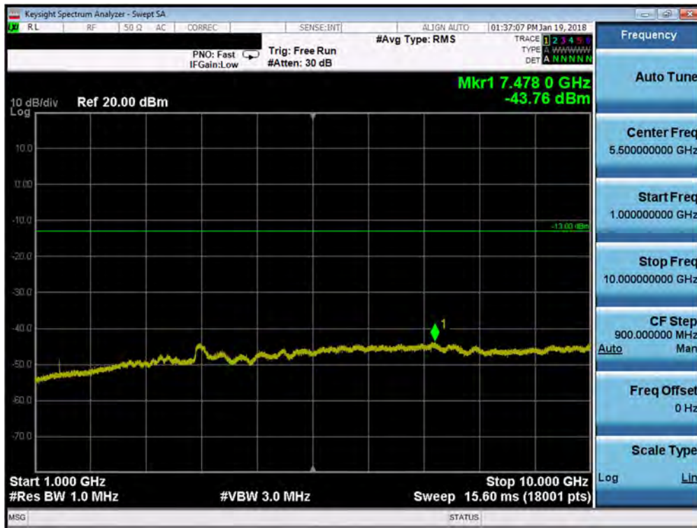
Plot 7-43. Conducted Spurious Plot (Band 12 - 10.0MHz QPSK - RB Size 1, RB Offset 0 - Low Channel)
