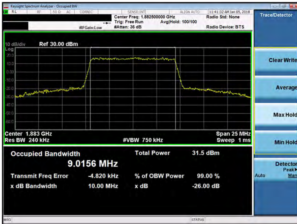
Plot 7-36. Occupied Bandwidth Plot (Band 2/25 - 10.0MHz 16-QAM - Full RB Configuration)
