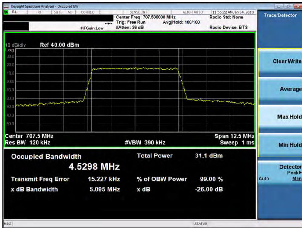
Plot 7-6. Occupied Bandwidth Plot (Band 12 - 5.0MHz 16-QAM - Full RB Configuration)
