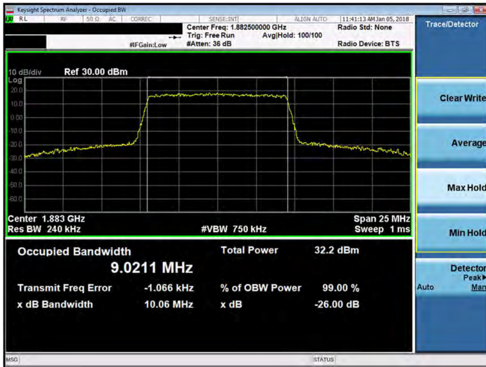
Plot 7-35. Occupied Bandwidth Plot (Band 2/25 - 10.0MHz QPSK - Full RB Configuration)
