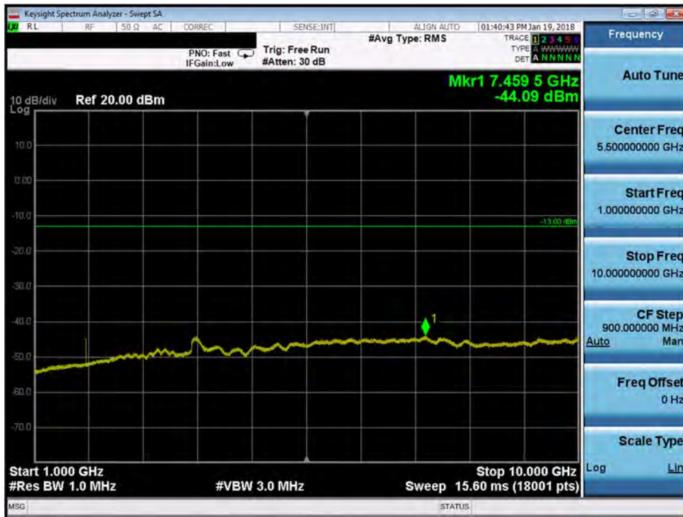
Plot 7-49. Conducted Spurious Plot (Band 12 – 10.0MHz QPSK - RB Size 1, RB Offset 0 - High Channel)
