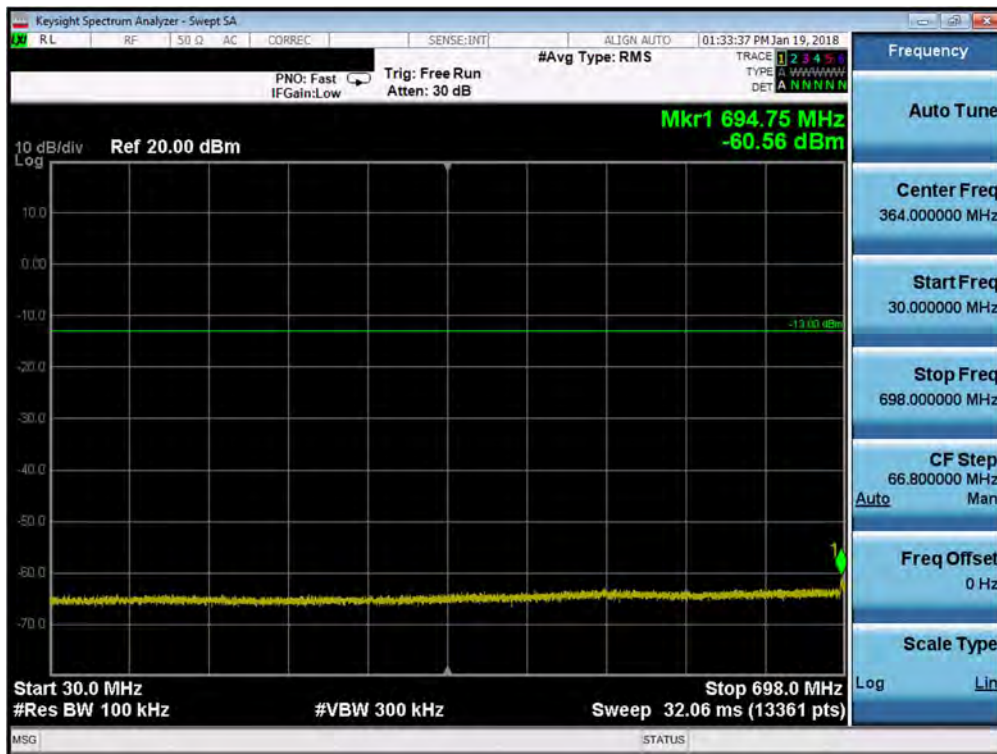
Plot 7-44. Conducted Spurious Plot (Band 12 - 10.0MHz QPSK - RB Size 1, RB Offset 0 - Mid Channel)
