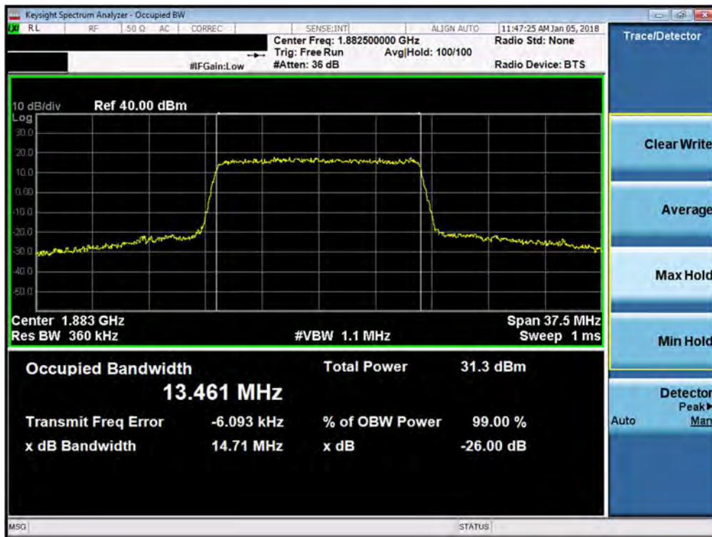
Plot 7-38. Occupied Bandwidth Plot (Band 2/25 - 15.0MHz 16-QAM - Full RB Configuration)
