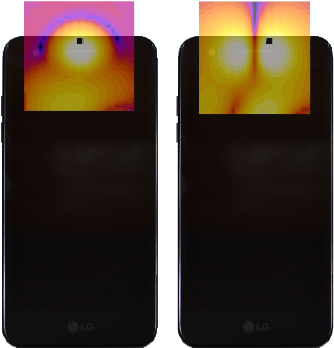
Figure 13-3 T-Coil Scan Overlay Magnetic Field Distributions
