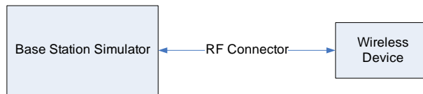
Figure 9-3 Power Measurement Setup
