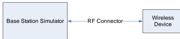
Figure 9-2 Power Measurement Setup
