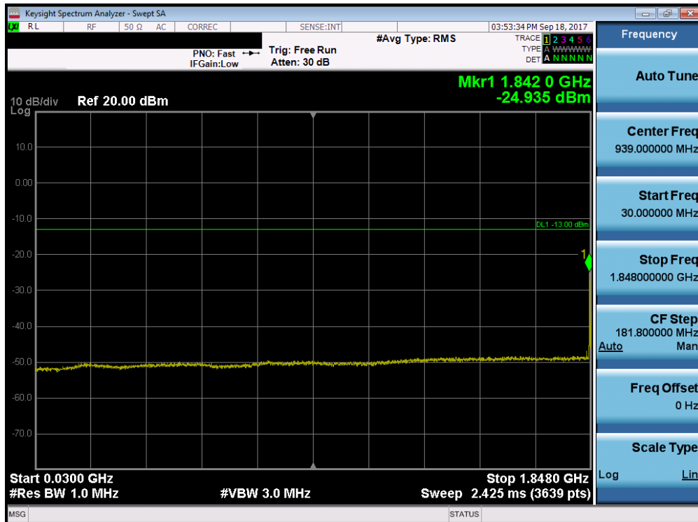
Plot 7-70. Conducted Spurious Plot (Band 2 - 10.0MHz QPSK - RB Size 1, RB Offset 0 - Low Channel)
