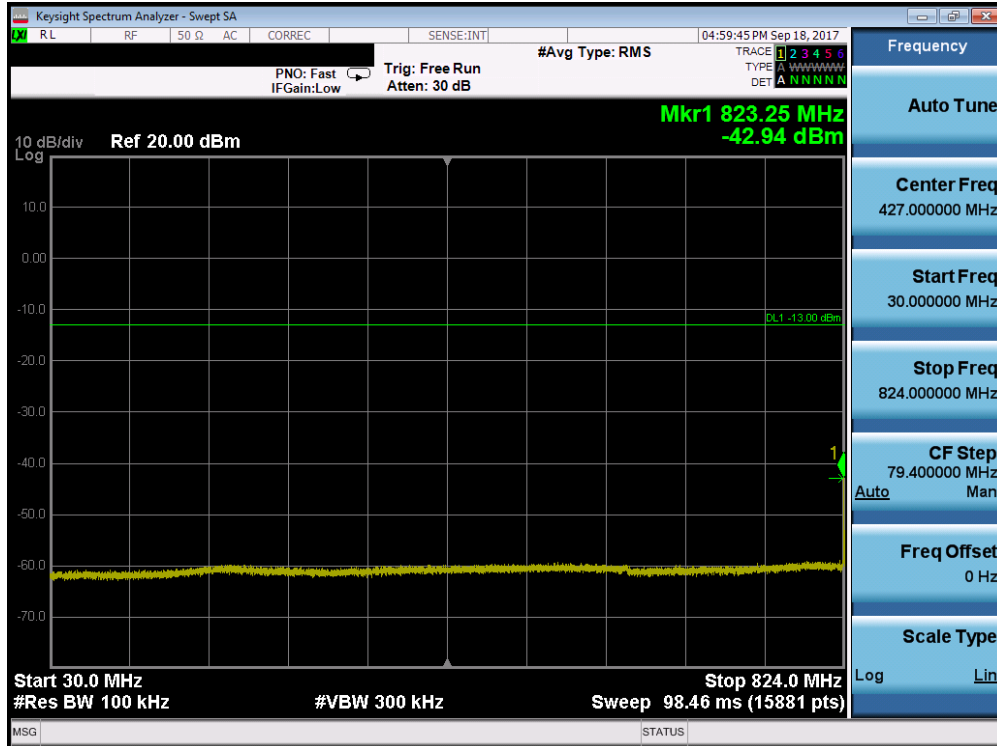
Plot 7-55. Conducted Spurious Plot (Band 5 - 10.0MHz QPSK - RB Size 1, RB Offset 0 - Mid Channel)
