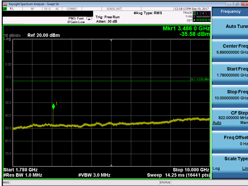
Plot 7-65. Conducted Spurious Plot (Band 66/4 - 5.0MHz QPSK - RB Size 1, RB Offset 0 - Mid Channel)
