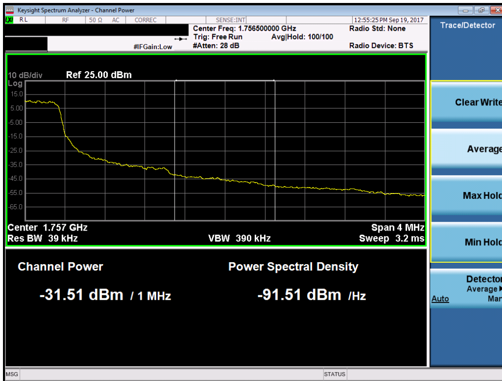
Plot 7-99. . Upper Extended Band Edge Plot (Band 4 - 1.4MHz QPSK - Full RB Configuration)
