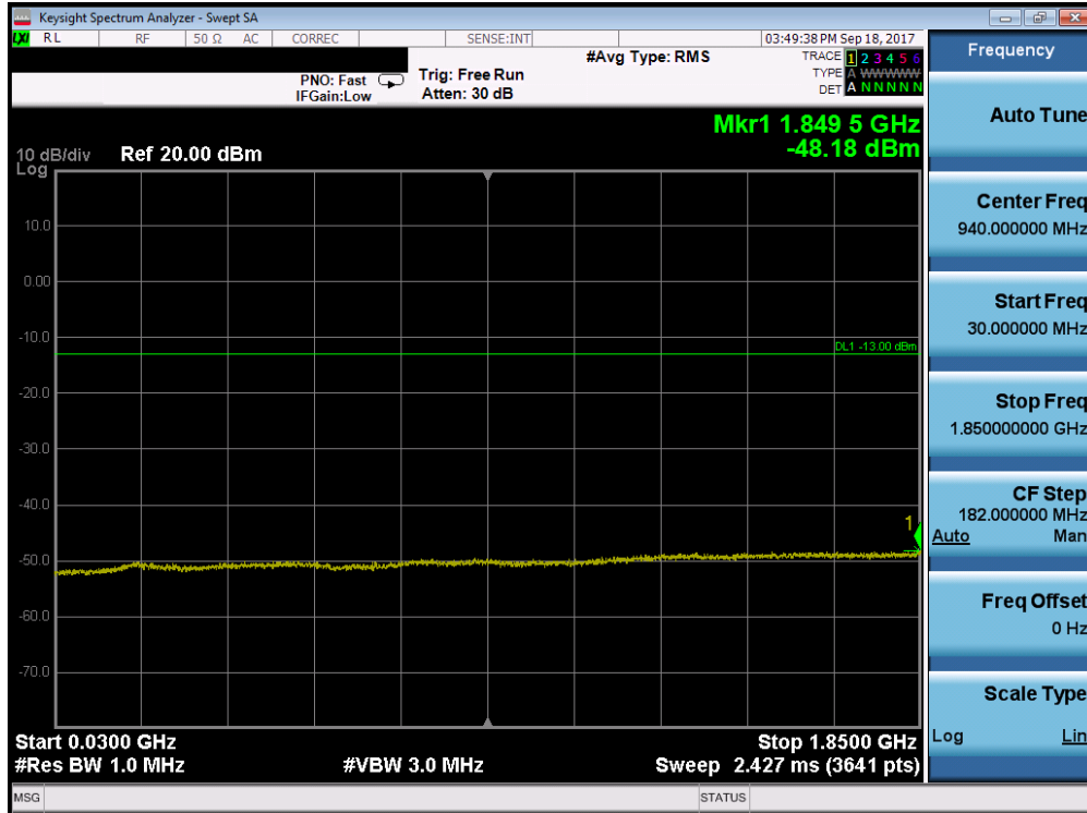
Plot 7-73. Conducted Spurious Plot (Band 2 - 10.0MHz QPSK - RB Size 1, RB Offset 0 - Mid Channel)
