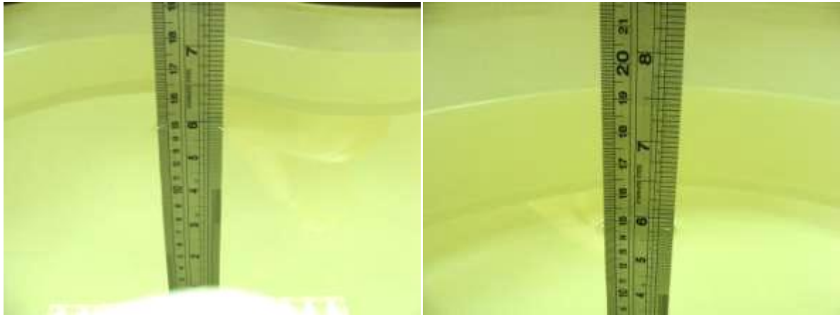
Photo of Liquid Height for Head SAR
